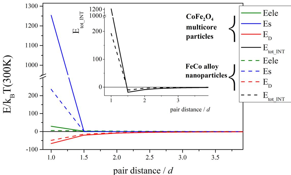
Fig. 2 Calculated reduced electrostatic  $E_{ele}$ , steric  $E_s$  and dipolar  $E_D$  interaction energy versus pair distance for multicore CFO particles (solid lines) and FeCo alloy nanoparticles (dashed lines). Inset: The corresponding total interaction energy  $E_{tot\_INT}$  versus pair distance. The pair distance is calculated in units of particle size  $d$ .
