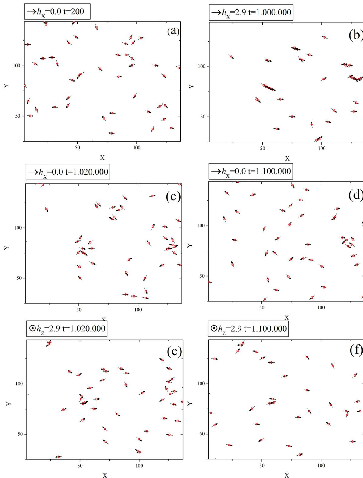
**Fig. 4** Snapshots of the coated FeCo alloy nanoparticles' configurations: (1) at the beginning of the process when the particles are randomly placed in the fluid (a), (2) under a magnetic field  $h_x = 2.9$  (b), (3) when switching off the field  $h_x = 0.0$  (c) and (d) and (4) when applying the field out-of-plane  $h_z = 2.9$  (e) and (f). The spin direction is indicated by the black arrows. The  $X$  and  $Y$  axes are calculated in units of particle size  $d = 10$  nm and the time in MCS.
