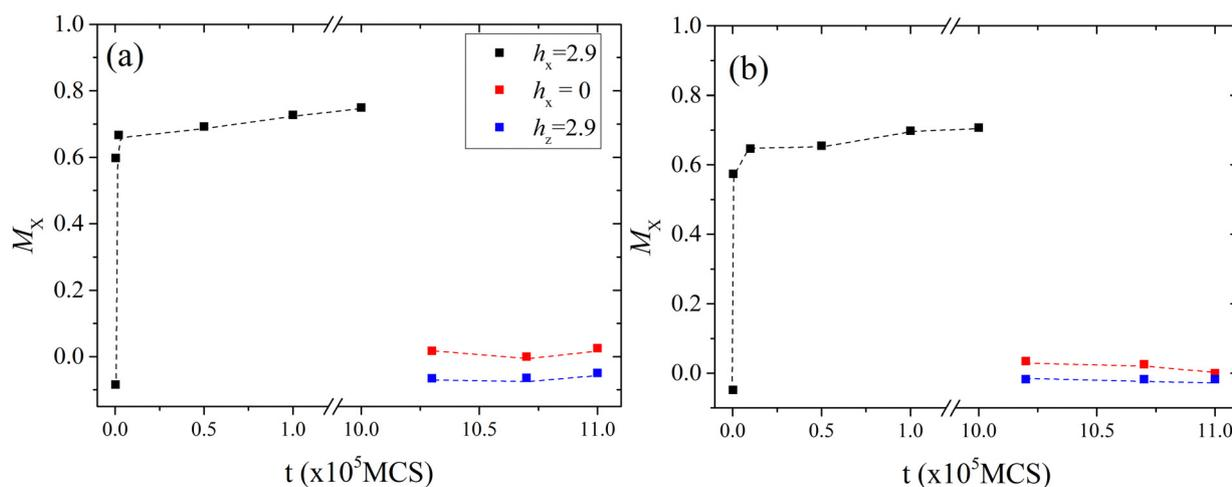
Fig. 6 The time dependence of the calculated in-plane mean magnetization  $M_x$  when the field is applied in-plane (black) and then it is turned off (red) or when the field is applied out-of-plane (blue): (a) coated CFO multicore particles (FF1) and (b) coated FeCo alloy nanoparticles in the fluid (FF2).
