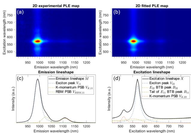
**Fig. 1** (a) Experimental PLE map from a (6, 5) sample sorted according to the methods described in ref. 4. (b) Fitted PLE map for this sample. (c) Emission lineshape with each of its components as explained in the text. (d) Excitation lineshape with each of its components as explained in the text.
