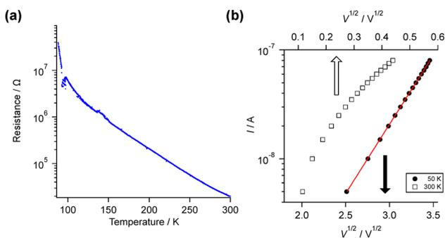
Fig. 3 Temperature-dependent electrical conduction measurement of  $C_{60}$  nanowires. (a) Electrical resistance of  $C_{60}$  nanowires plotted against temperature. (b)  $I_{DS}$ - $V_{DS}$  curves at different temperatures at 50 and 300 K. These measurements were fixed for  $W = 200 \mu\text{m}$  and  $f = 1 \times 10^{10} \text{cm}^{-2}$ .
