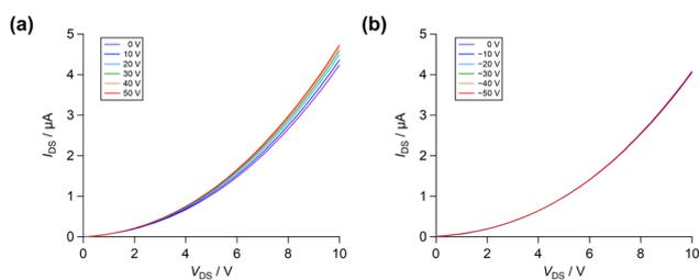
**Fig. 5** FET characteristics of  $\text{C}_{60}$  nanowires.  $I$ – $V$  characteristics ( $I_{\text{DS}}$  vs.  $V_{\text{DS}}$ ) at (a)  $V_{\text{G}} = 0$  to  $50 \text{ V}$  and (b)  $V_{\text{G}} = 0$  to  $-50 \text{ V}$  in a step of  $10 \text{ V}$ . These measurements were fixed for  $W = 1500 \mu\text{m}$  and  $f = 1 \times 10^{11} \text{ cm}^{-2}$ .
