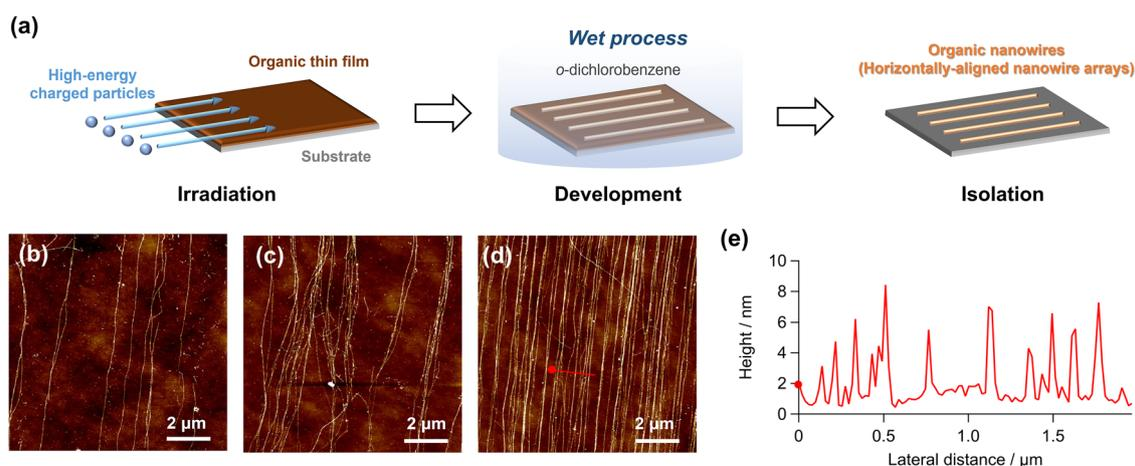
**Fig. 1** Fabrication of horizontally aligned nanowire arrays by high-energy charged particle irradiation. (a) Schematic illustration of horizontally – aligned C<sub>60</sub> nanowire arrays *via* the STLiP method. (b)–(d) AFM images of horizontally aligned nanowire arrays at a fluence ( $f$ ) of (b)  $1 \times 10^9$  cm<sup>-2</sup>, (c)  $1 \times 10^{10}$  cm<sup>-2</sup>, and (d)  $1 \times 10^{11}$  cm<sup>-2</sup>. (e) Height profile along the red line in Fig. 1(d).
