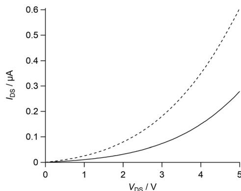
**Fig. 6** Electrical conduction property changes due to gas molecule adsorption.  $I$ – $V$  characteristics ( $I_{\text{DS}}$  vs.  $V_{\text{DS}}$ ), at  $V_{\text{G}} = 0$ , before (dotted line) and after (solid line) adsorption of nitrobenzene. These measurements were fixed for  $W = 1500 \mu\text{m}$  and  $f = 1 \times 10^{11} \text{ cm}^{-2}$ .
