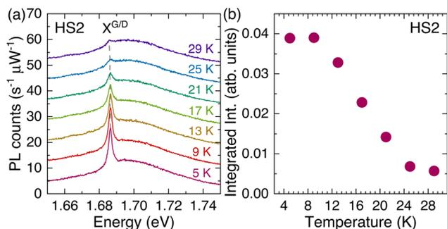
Fig. 4 (a) The temperature dependent photoluminescence spectra of the hBN/WSe<sub>2</sub>/CrCl<sub>3</sub>/hBN heterostructure (HS2) in range of temperatures 5–29 K. Spectra were shifted vertically for clarity. (b) The integrated intensity of the gray/dark exciton X<sup>G/D</sup> resonance is shown as a function of temperature.
