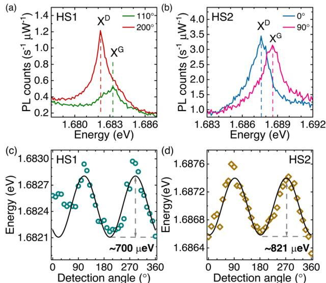
Fig. 3 Low temperature ( $T = 5$  K) photoluminescence spectra of the gray/dark exciton resonance (X<sup>G/D</sup>) recorded for two orthogonal linear polarizations measured for two hBN/WSe<sub>2</sub>/CrCl<sub>3</sub>/hBN heterostructures (HS): (a) HS1 and (b) HS2. The corresponding linear polarization dependence of the gray/dark exciton energy is presented for (c) HS1 and (d) HS2 samples. The solid black curves demonstrate the results of the least square fitting method using eqn (1).
