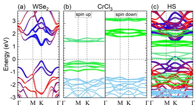
**Fig. 2** The element-projected band structure of (a) WSe<sub>2</sub> monolayer, (b) CrCl<sub>3</sub> ML, and (c) WSe<sub>2</sub>/CrCl<sub>3</sub> heterostructure. The atomic projection is color-coded as follows: W (blue), Se (red), Cr (light-blue), and Cl (light-green). In the heterostructure (HS) case, the lattice of WSe<sub>2</sub> monolayer was stretched to match the Brillouin zone high symmetry points between both materials for ease of comparison.
