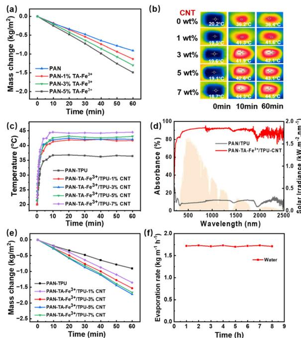
Fig. 4 (a) Water evaporation performance of single PAN-TA-Fe<sup>3+</sup> fibrous membrane. (b) Infrared thermal images and (c) temperature of the top surface of PAN-TA-Fe<sup>3+</sup>/TPU-CNT fibrous membrane versus time with different CNT contents. (d) Solar spectrum irradiance (AM 1.5G) and the absorption spectrum of PAN/TPU and PAN-TA-Fe<sup>3+</sup>/TPU-CNT fibrous membrane. (e) Water evaporation performance and (f) stability of PAN-TA-Fe<sup>3+</sup>/TPU-CNT fibrous membrane.
