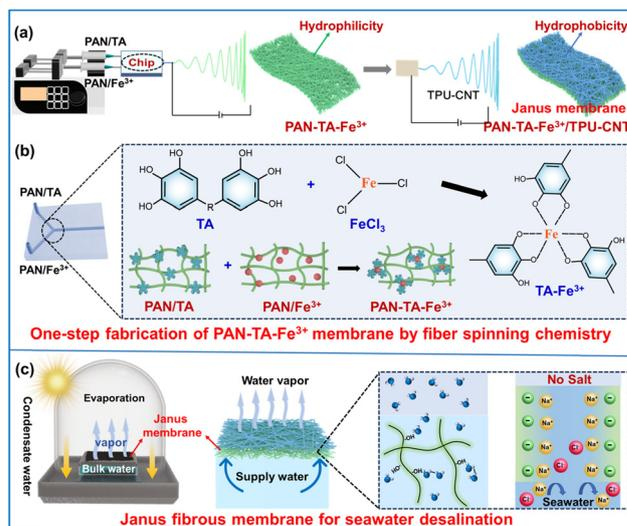
Fig. 1 (a) Schematic illustration of the fabrication of the PAN–TA–Fe<sup>3+</sup>/TPU–CNT Janus fibrous membrane via continuous microfluidic electrospinning. (b) Schematic illustration of the *in situ* chemical reaction between TA and Fe<sup>3+</sup> in microfluidic chip during spinning process. (c) Schematic illustration of the water evaporation process and mechanism.
