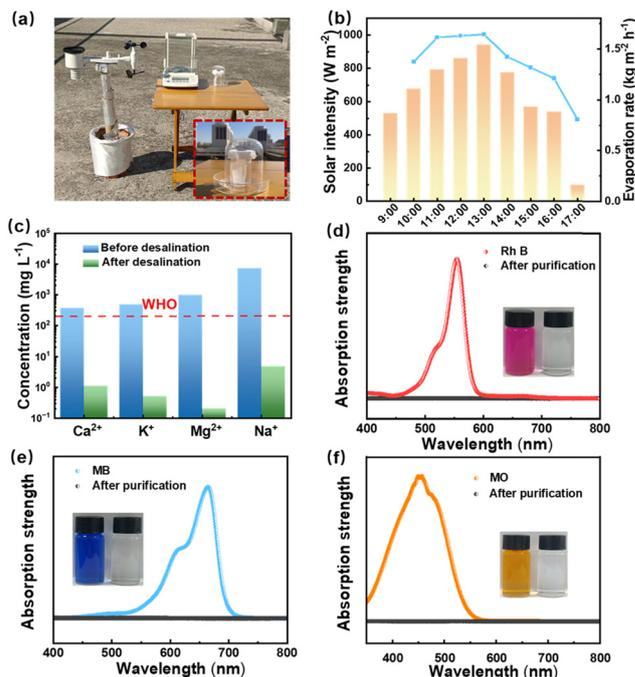
Fig. 6 (a) Digital photograph of an outdoor evaporation device. (b) Outdoor seawater evaporation performance of PAN-TA-Fe<sup>3+</sup>/TPU-CNT Janus fiber membrane. (c) Ca<sup>2+</sup>, K<sup>+</sup>, Mg<sup>2+</sup> and Na<sup>+</sup> concentration of the seawater before and after desalination. (d)–(f) UV-Vis spectroscopy before and after purification of Rh B, MB and MO solution.
