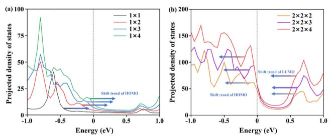
Fig. 3 Projected density of states (PDOS) of SMWs. (a) PDOS of quasi-1D W@Cu<sub>12</sub> SMWs. (b) PDOS of quasi-1D bundle-like W@Cu<sub>12</sub> SMWs. The gray dashed line represents the Fermi level. The arrows indicate the tendency of the HOMO and the LUMO to shift in energy as the length of the SMWs increases.
