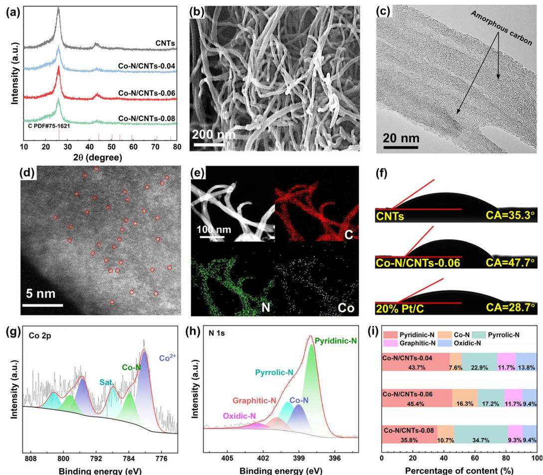
Fig. 2 (a) XRD patterns of CNTs, Co-N/CNTs-0.04, Co-N/CNTs-0.06, and Co-N/CNTs-0.08. (b) SEM image, (c) TEM image, and (d) AC-STEM image of Co-N/CNTs-0.06. (e) The corresponding elemental mapping images of Co-N/CNTs-0.06. (f) Contact angle of CNTs, Co-N/CNTs-0.06 and 20% Pt/C. (g) Co 2p and (h) N 1s XPS spectra of Co-N/CNTs-0.06. (i) The relative proportion of different types of N species on the surface of Co-N/CNTs-0.04, Co-N/CNTs-0.06, and Co-N/CNTs-0.08.
