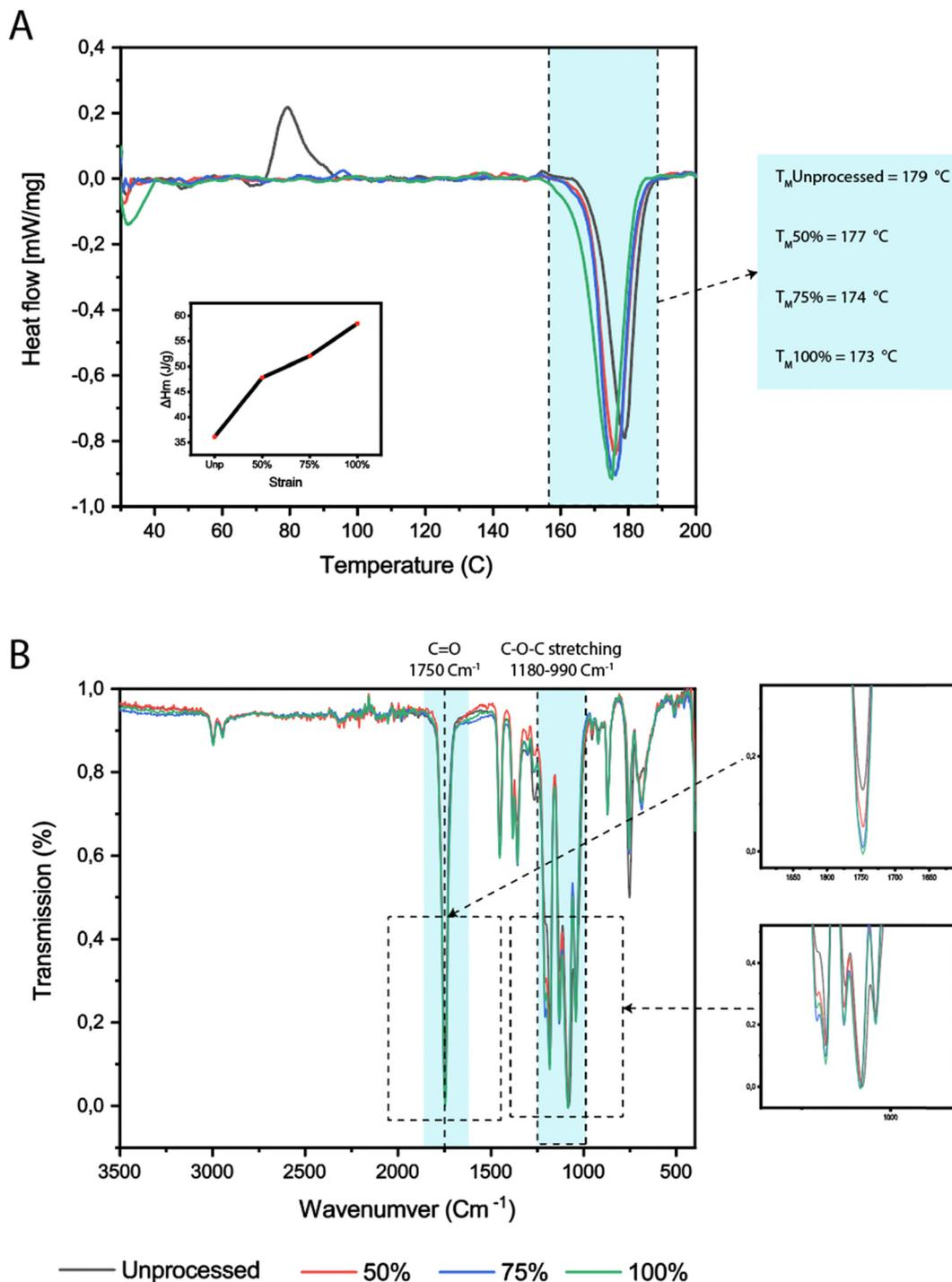
Fig. 2 (A) DSC data of the unprocessed and differently strained films. The melting temperature ( $T_m$ ) is highlighted with a blue border, and the melting temperatures corresponding to each strain are indicated beneath the figure. (inset) Heat of melting ( $\Delta H_m$ ) plotted as a function of strain percentage, used to determine crystallinity content. (B) FTIR data of the unprocessed and differently strained films. (inset) Enlarged views of the regions are indicated by dashed boxes.
