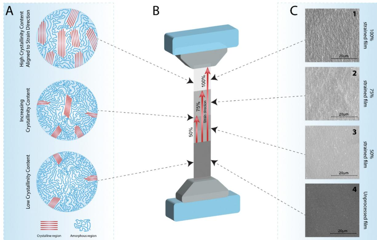
**Fig. 1** (A) Illustration of the polymer orientation and the corresponding changes in crystallinity due to this post-processing of casted film. (B) Illustration of the Uniaxial stretching post-processing method. (C) SEM images of the unprocessed and strained films.
