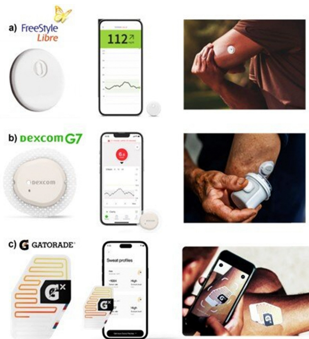
Fig. 2 Examples of commercial wearable biosensors for continuous health monitoring. (a) FreeStyle Libre by Abbott for real-time blood glucose monitoring. 39 (b) Dexcom G7 by Dexcom for advanced continuous glucose tracking. 40 (c) Gx Sweat Patch by Epicore Biosystems (Gatorade) for hydration and electrolyte analysis through sweat. 41,42
