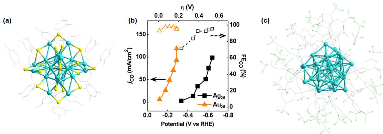
Fig. 3 (a) Structural architecture of Ag<sub>25</sub> NC. H atoms are omitted for the clarity. Color legend: Ag, aqua; S, yellow; and C, gray. (b) Comparison of ECO<sub>2</sub>R data between [Au<sub>25</sub>]<sup>-</sup> and Ag<sub>25</sub> NCs. Reproduced with permission from ref. 85. Copyright 2022 Americal Chemical Society. (c) Structural architecture of alkynyl-protected Ag<sub>32</sub> NC. H atoms are omitted for the clarity. Color legend: Ag, aqua; F, green; and C, gray.
