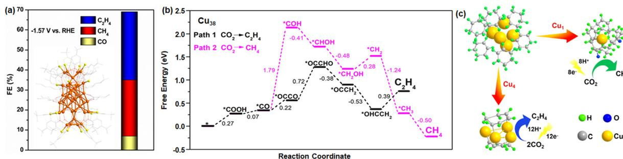
Fig. 8 (a) Structural architecture of Cu<sub>38</sub> NC and FE. H atoms are omitted for the clarity. Color legend: Cu, brown; S, yellow; O, red; and C, gray. (b) Theoretical reaction mechanism through free energy profile. Reproduced with permission from ref. 109. Copyright 2024 Americal Chemical Society. (c) Comparison in ECO<sub>2</sub>R product when Cu NCs embedded on MWCNT. Reproduced with permission from ref. 110. Copyright 2021 Americal Chemical Society.
