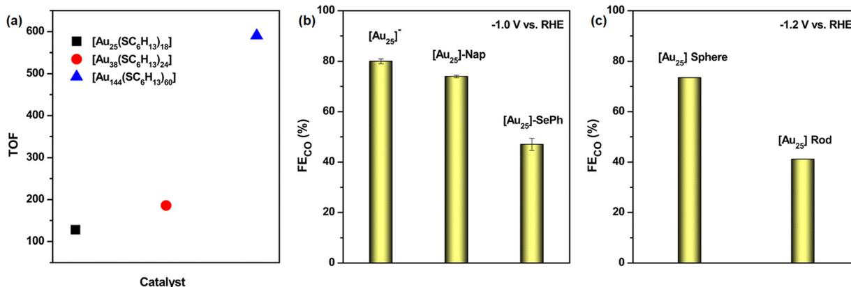
Fig. 2 (a) TOF comparison in  $-0.56$  V vs. RHE among  $\text{Au}_{25}(\text{SC}_6\text{H}_{13})_{18}$ ,  $\text{Au}_{38}(\text{SC}_6\text{H}_{13})_{24}$ , and  $\text{Au}_{144}(\text{SC}_6\text{H}_{13})_{60}$  NCs. (b) Comparison of  $\text{FE}_{\text{CO}}$  among of  $[\text{Au}_{25}]^-$  NCs with ligand variation. (c) Comparison of  $\text{FE}_{\text{CO}}$  in  $[\text{Au}_{25}]^-$  NCs depending on their morphology.
