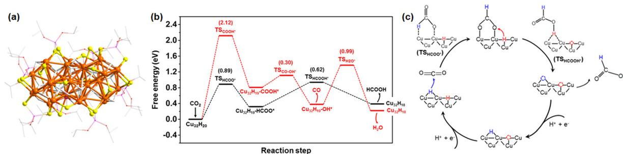
Fig. 4 (a) Structural architecture of Cu<sub>32</sub> NC. H atoms are omitted partially for the clarity. Color legend: Cu, brown; S, yellow; P, magenta stick; O, red stick; C, gray stick; and H, white. (b) Theoretical Free energy calculations for CO and HCOOH formation by Cu<sub>32</sub> NC. (c) Mechanistic pathway for HCOOH formation form CO<sub>2</sub> reduction. Reproduced with permission from ref. 100. Copyright 2017 American Chemical Society.
