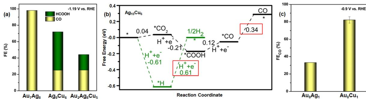
Fig. 9 (a) Comparison of FE series of among alkynyl-protected M<sub>15</sub> alloy NCs. (b) Theoretical reaction mechanism through free energy profile by using Ag<sub>15</sub>Cu<sub>6</sub> NC as catalyst. Reproduced with permission from ref. 123. Copyright 2023 Americal Chemical Society. (c) Comparison of FE with different M<sub>9</sub> alloy NCs.
