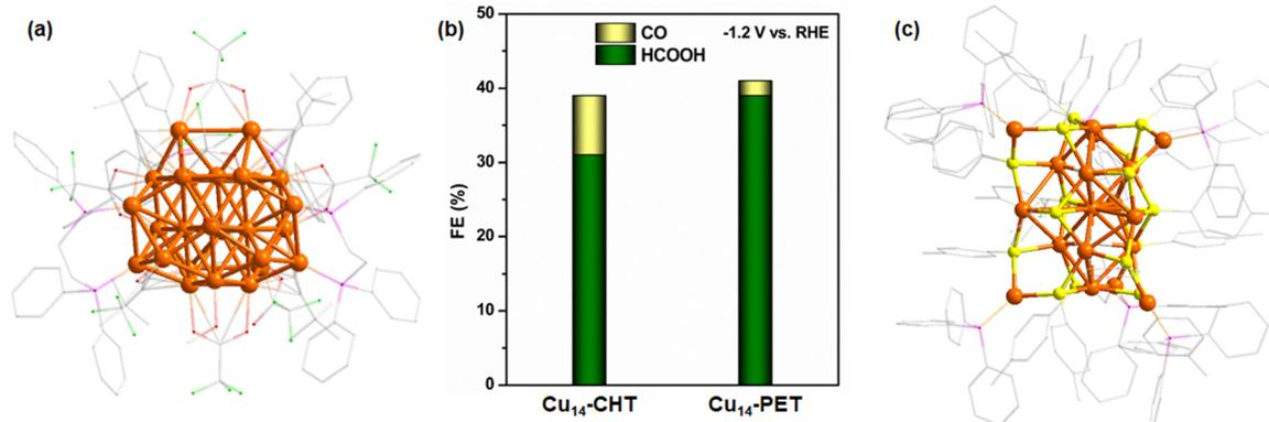
Fig. 5 (a) Structural architecture of Cu<sub>26</sub> NC. H atoms are omitted for the clarity. Color legend: Cu, brown; P, magenta stick; Cl, green stick; O, red stick; and C, gray stick. (b) Comparison of FE between Cu<sub>14</sub>-CHT and Cu<sub>14</sub>-PET NCs. (c) Structural architecture of Cu<sub>26</sub> NC. H atoms are partially omitted for the clarity. Color legend: Cu, brown; P, magenta stick; C, gray stick; and H, white.
