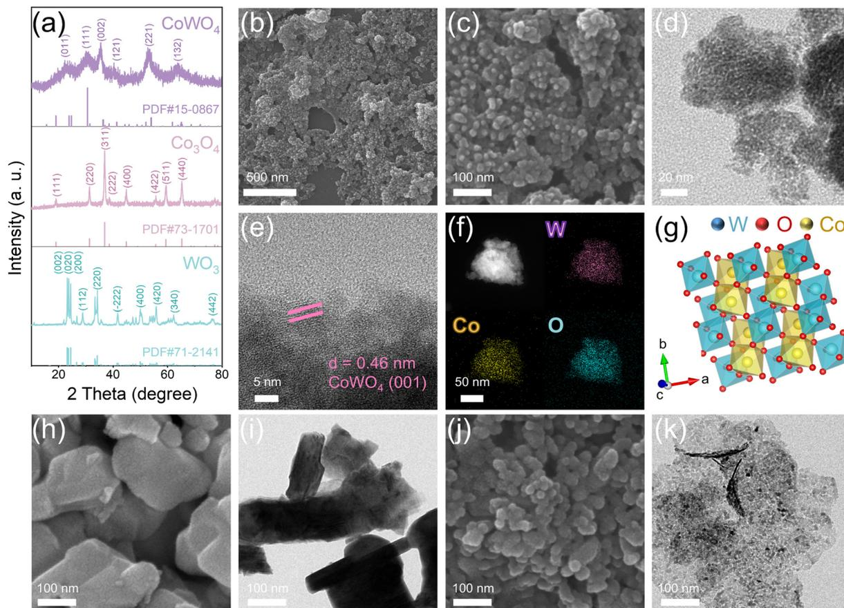
Fig. 2 (a) XRD patterns of  $\text{CoWO}_4$ ,  $\text{Co}_3\text{O}_4$ , and  $\text{WO}_3$ ; (b) and (c) SEM images of  $\text{CoWO}_4$ ; (d) TEM image of  $\text{CoWO}_4$ ; (e) HR-TEM image of  $\text{CoWO}_4$ ; (f) HAADF-STEM image of  $\text{CoWO}_4$  and the corresponding EDS elemental maps of W, Co, and O; (g) microscopic atomic structure modeling of  $\text{CoWO}_4$ ; (h) and (i) SEM and TEM images of  $\text{WO}_3$ ; (j) and (k) SEM and TEM images of  $\text{Co}_3\text{O}_4$ .
