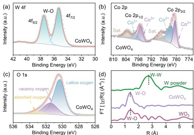
Fig. 3 High resolution XPS spectra of (a) W 4f, (b) Co 2p, and (c) O 1s for CoWO<sub>4</sub>. (d) Fourier transform magnitudes in *R* space of the W L<sub>3</sub>-edge for WO<sub>3</sub>, CoWO<sub>4</sub>, and W powder.
