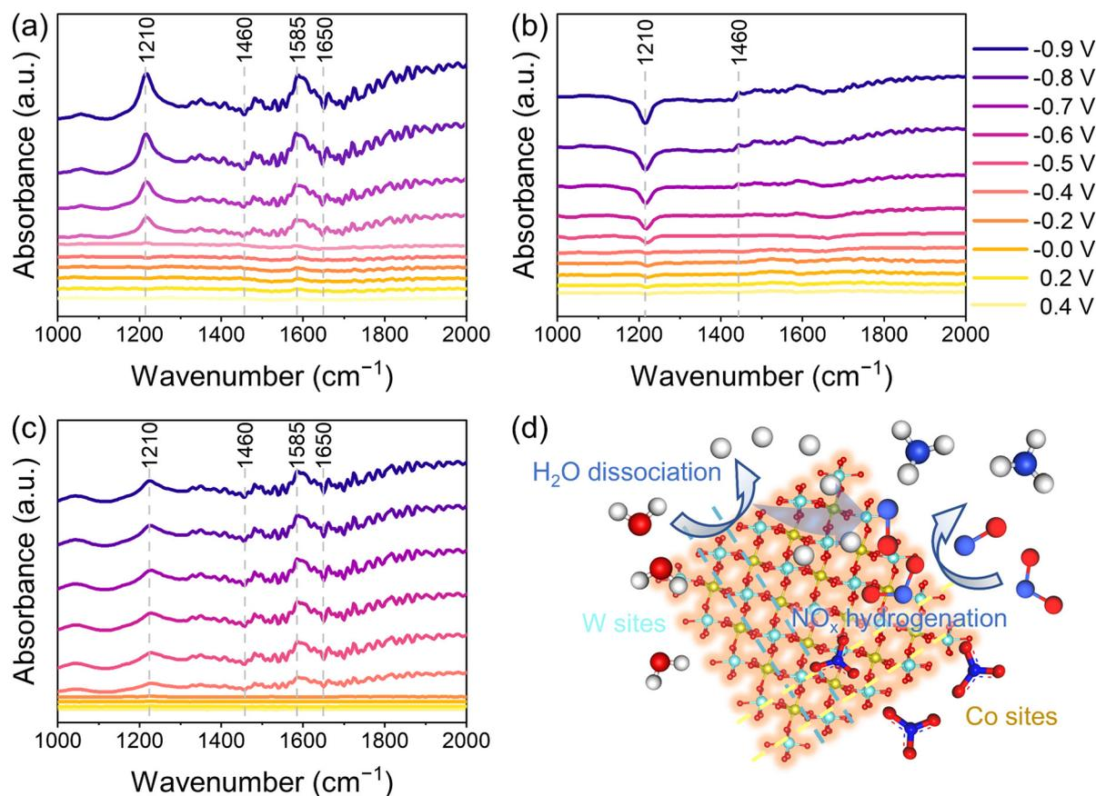
Fig. 6 *In situ* FT-IR spectra of (a)  $\text{CoWO}_4$ , (b)  $\text{WO}_3$ , and (c)  $\text{Co}_3\text{O}_4$  at different applied potentials. (d) Proposed catalytic reaction mechanism for  $\text{NH}_3$  formation on  $\text{CoWO}_4$ .
