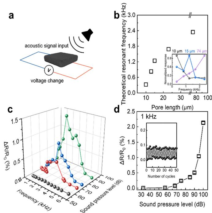
**Fig. 4** (a) Schematic of the rGO/DNA aerogel-based acoustic sensing test. (b) Theoretical resonant frequency of rGO/DNA aerogels with different pore lengths. Inset: Normalized response of rGO/DNA aerogel-based acoustic sensors with pore sizes of 10  $\mu\text{m}$ , 15  $\mu\text{m}$ , and 74  $\mu\text{m}$ . (c) Resistance response for different frequencies and sound pressure levels. (d) Resistance response at 1 kHz vs. sound pressure level. Inset: Repeatability test at 1 kHz under 50 cycles.
