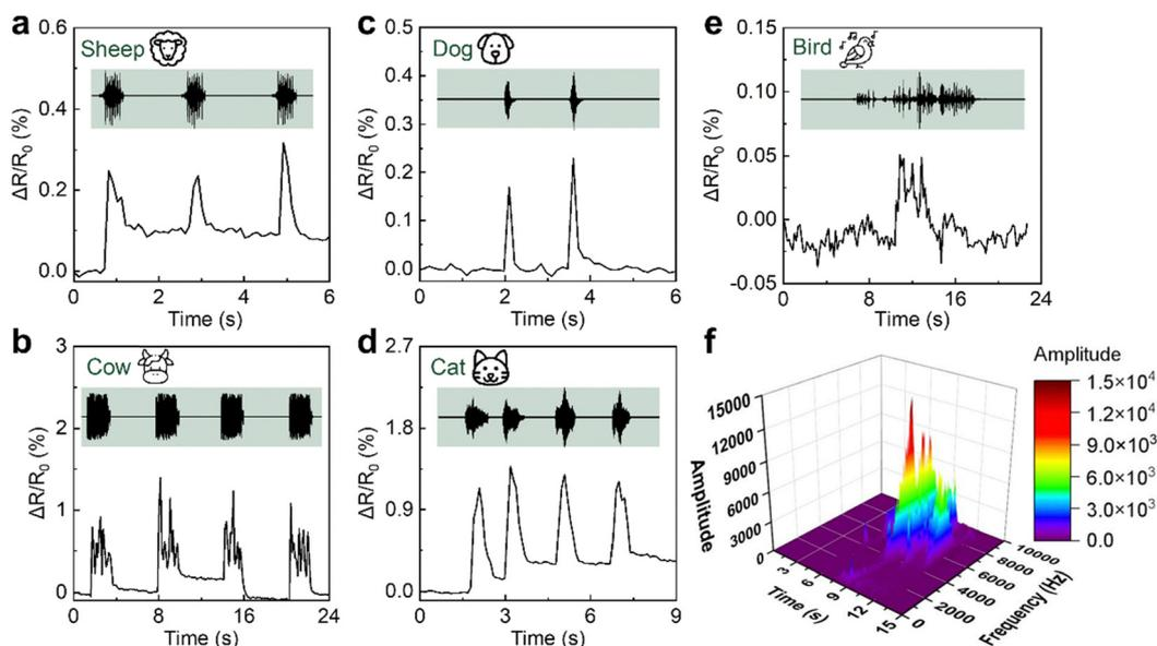
**Fig. 5** Resistance response of the rGO/DNA aerogel-based acoustic sensor in response to the audio signals of animal sounds: (a) a sheep, (b) a cow, (c) a dog, (d) a cat, and (e) a bird. (f) The short-time Fourier transform analysis of the bird's chirp.
