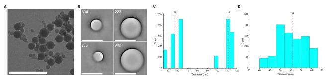
Fig. 4 PS Mixed system (A) raw example micrograph, scale bar 500 nm (B) example 2D classes including the class population numbers, scale bar 100 nm (C) histogram of class average sizes when analysing both large and small systems together with a histogram class binning of 4 nm (D) histogram of class average sizes of PS50 NPs from the same mixed system, histogram class binning of 4 nm.
