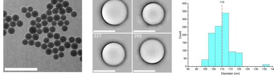
Fig. 3 2D-CA of PS100 polystyrene NPs: (A) example of a raw micrograph used for analysis (B) example of the resulting 2D classes including the class population numbers. (C) Histogram showing the size distribution as reconstructed from 11 class averages, yielding a number average of 110 nm for the PS100 NPs. Histogram binning is 4 nm. Scale bars (A) 500 nm and (B) 100 nm.
