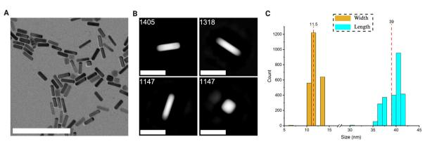
Fig. 6 Au Nanorod system (A) raw example micrograph, scale bar 250 nm (B) example 2D classes including the class population numbers, scale bar 40 nm (C) histogram of class average sizes when analysing both width and length of the nanorods with a histogram class binning of 1 nm.
