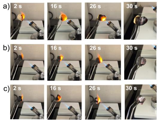
Fig. 5 Flammability test of foams. Alginate (a), 1%Ti<sub>3</sub>C<sub>2</sub>T<sub>x</sub>-alginate (b), and 5%Ti<sub>3</sub>C<sub>2</sub>T<sub>x</sub>-alginate (c) foams subjected to a butane torch flame; snapshots were taken after 2, 16, 26, and 30 s.
