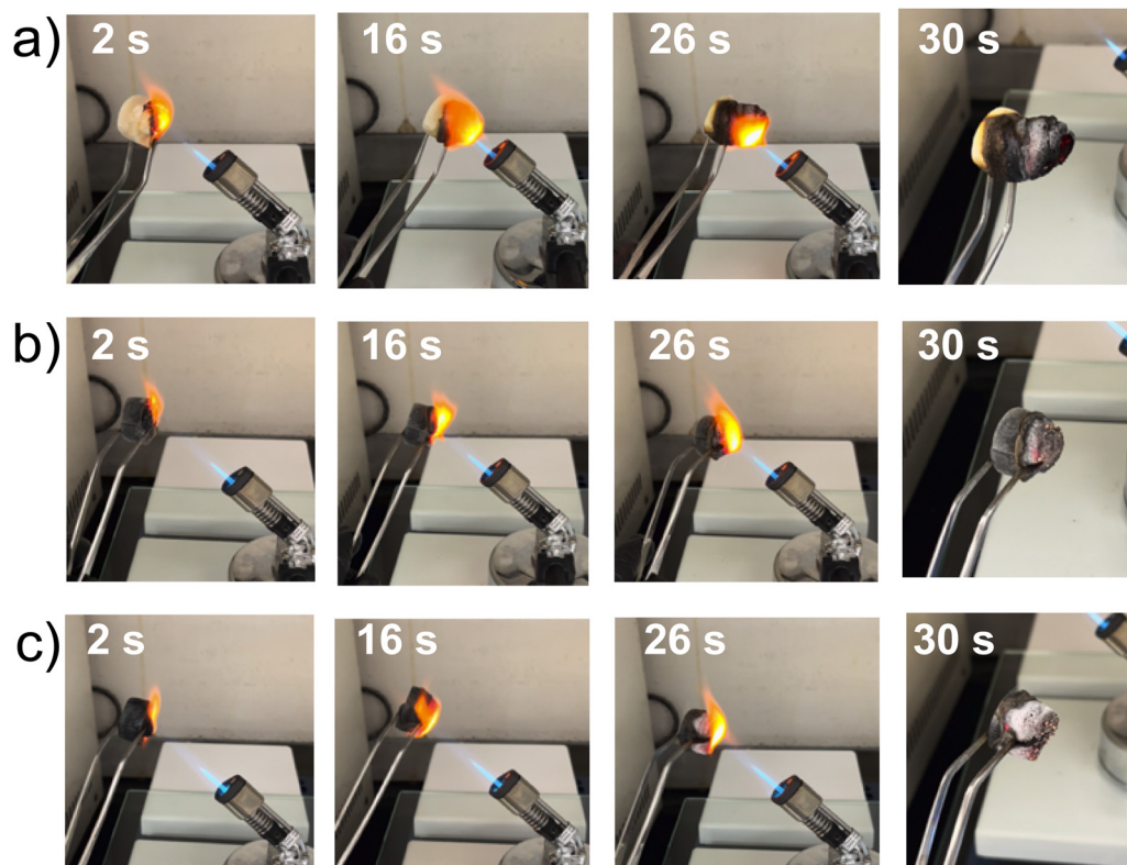
Fig. 5 Flammability test of foams. Alginate (a), 1% \text{Ti}_3\text{C}_2\text{T}_x -alginate (b), and 5% \text{Ti}_3\text{C}_2\text{T}_x -alginate (c) foams subjected to a butane torch flame; snapshots were taken after 2, 16, 26, and 30 s.
