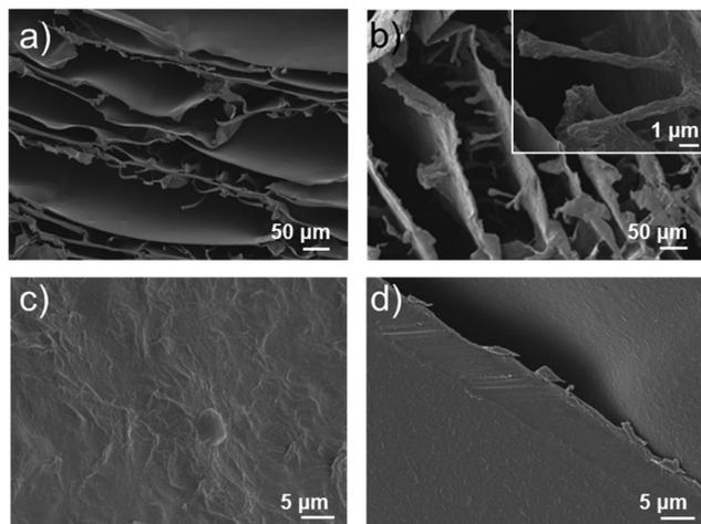
Fig. 2 Morphology of the foams. SEM cross-sectional images of an alginate (a) and 5% $\text{Ti}_3\text{C}_2\text{T}_x$ -alginate foam; inset shows details at higher magnification (b). Images of the foam wall surfaces of 5% $\text{Ti}_3\text{C}_2\text{T}_x$ -alginate and alginate foams (c), (d).
