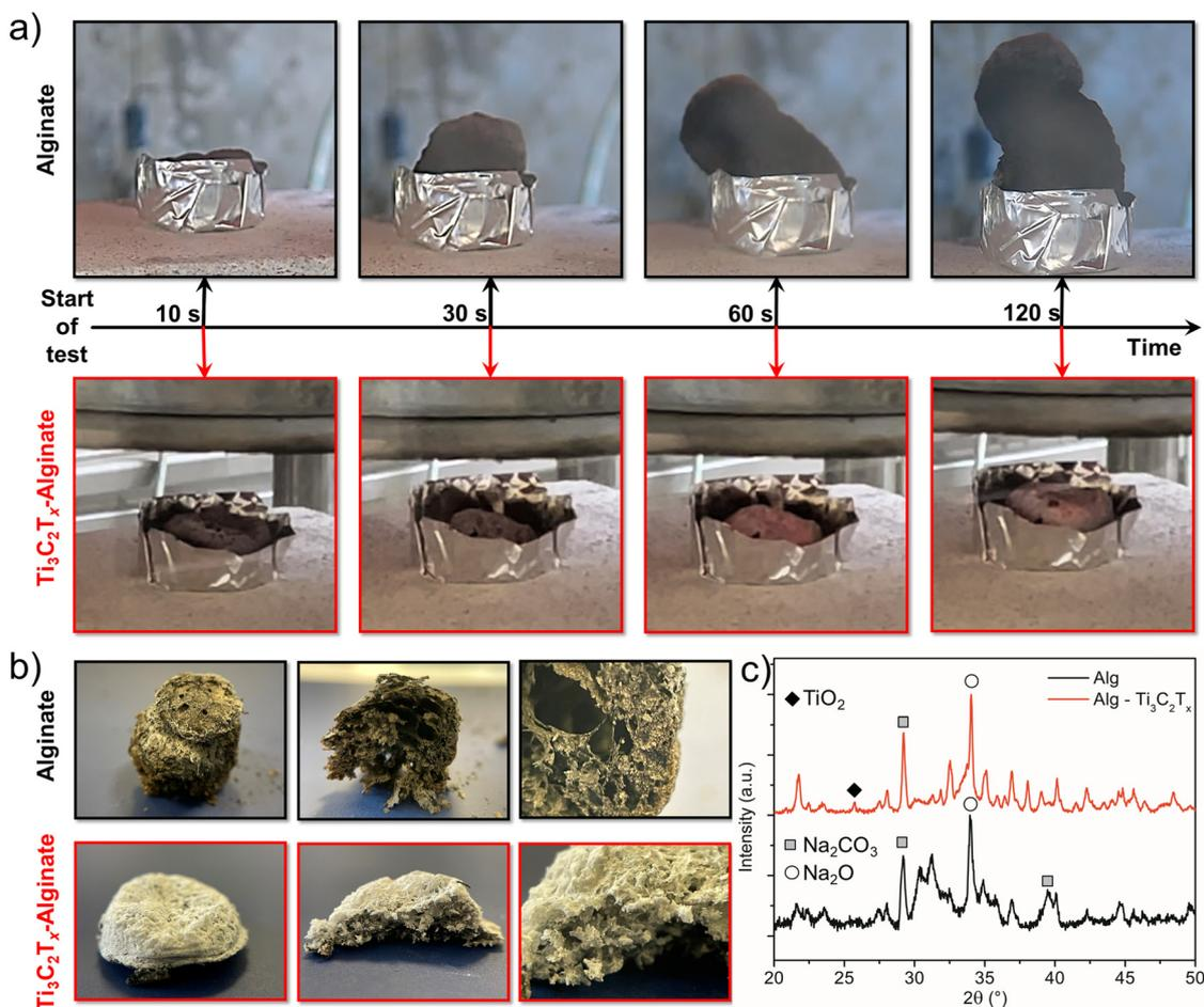
Fig. 6 Cone calorimetry tests of foams. Digital images of the foams during the tests (a) and after collecting the residues (b). XRD diffractograms of the residues of alginate and 5% $\text{Ti}_3\text{C}_2\text{T}_x$ -alginate (c).
