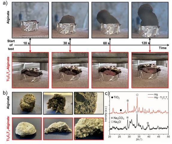
Fig. 6 Cone calorimetry tests of foams. Digital images of the foams during the tests (a) and after collecting the residues (b). XRD diffractograms of the residues of alginate and 5%Ti<sub>3</sub>C<sub>2</sub>T<sub>x</sub>-alginate (c).
