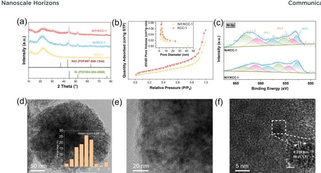
Fig. 2 (a) XRD patterns of Ni/KCC-1 and NiY/KCC-1 catalysts and KCC-1; (b) N<sub>2</sub> adsorption—desorption curves and pore width distributions of Ni/KCC-1 and NiY/KCC-1 catalysts; (c) XPS of Ni2p; (d)-(f) HR-TEM images and locally enlarged images of NiY/KCC-1.
