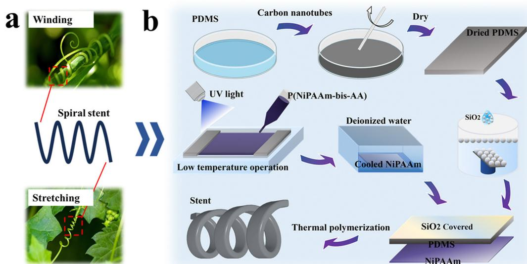
**Fig. 1** Schematic illustrations of the fabrication of the helical hydrogel fiber. (a) Drawing inspiration from the helical winding structures of natural vines, a Janus-featured, thermally responsive helical PDMS stent was designed; (b) a layered helical fiber comprising PNiPAAm inverse opal/PDMS was fabricated using the sandwich thermoplastic method.
