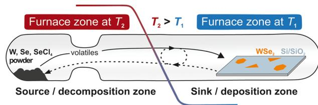
**Fig. 1** Concept of the experimental work-up of the CVT experiment using a two-chamber silica glass ampoule. Starting materials are placed on the source side ( $T_2$ ) and the  $\text{SiO}_2$ @Si(100) substrate is positioned on the sink side ( $T_1$ ), with  $T_2 > T_1$ . An applied temperature gradient is given as the red line.
