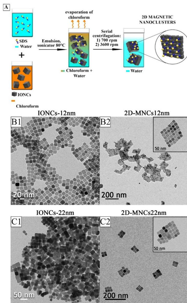
Fig. 1 (A) Schematic drawing illustrating the micro emulsion-based solvent evaporation technique used for controlled 2D ordering of IONCs. TEM images of (B1) as-synthesized IONCs of 12 nm in  $\text{CHCl}_3$  and (C1) as-synthesized IONCs of 22 nm in  $\text{CHCl}_3$  and corresponding (B2) 2D-MNCs12 nm and (C2) 2D-MNCs22 nm after emulsification with SDS deposited from water, after purification.
