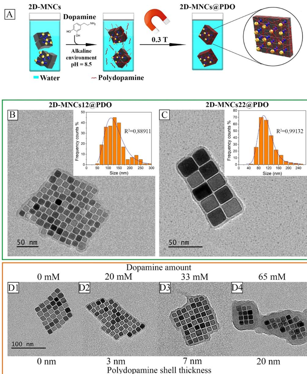
**Fig. 2** (A) General scheme showing the coating process of 2D-MNCs by PDO. TEM images of, (B) 2D-MNCs12 obtained after PDO polymerization (2D-MNCs12@PDO); inset – size distribution histogram of 2D-MNCs12@PDO; (C) 2D-MNCs22@PDO obtained from 2D-MNCs22 nm. Inset – size distribution histogram of 2D-MNCs22@PDO; (D) TEM images of 2D-MNCs12@PDO clusters, where we assess the PDO thickness on clusters as a function of dopamine solution concentrations; (D1) 0 mM, (D2) 20 mM, (D3) 32 mM and (D4) 65 mM.
