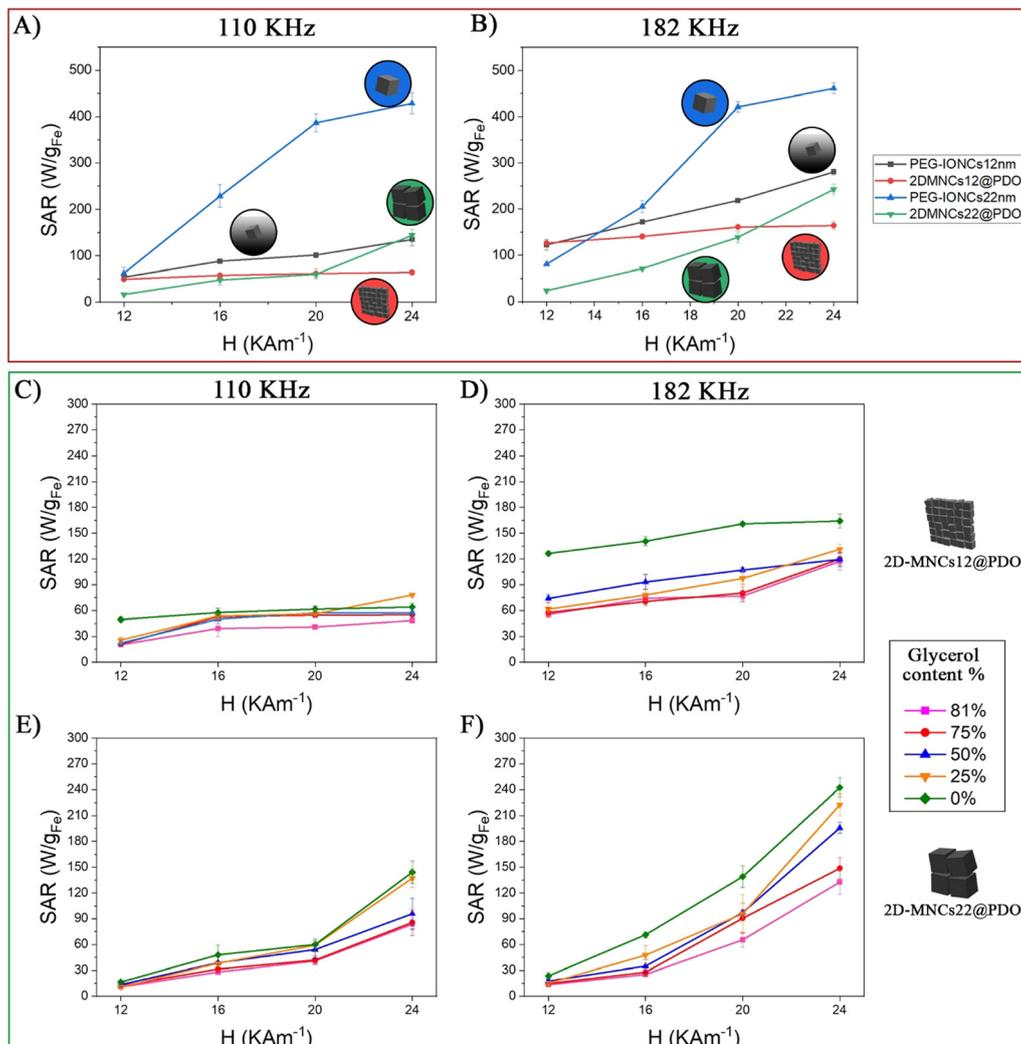
Fig. 7 Field dependence of the specific absorption rate (SAR) of (A) PEG-IONCs12 nm and 2D-MNCs12@PDO and (B) PEG-IONCs22 nm and 2D-MNCs22@PDO. SAR evolution vs. glycerol content (wt%) and  $\eta$ , measured at 12, 16, 20 and 24  $\text{kA m}^{-1}$  and 110 and 182 KHz for (C), (D) 2D-MNCs12@PDO and (E), (F) 2D-MNCs22@PDO.
