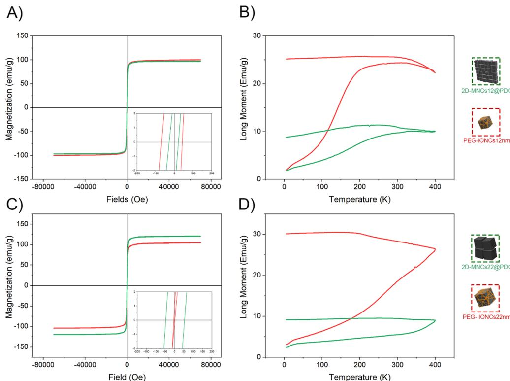
**Fig. 6** Normalized magnetization curves measured at RT for (A) 2D-MNCs12@PDO (green line), PEG-IONCs12 nm (red line) and (C) 2D-MNCs22@PDO (green line), PEG-IONCs22 nm (red line). The insets represent a detail of the low field region. Thermal dependence of the magnetization upon zero field cooling ( $H_{\text{meas}} = 50$  Oe) for (B) 2D-MNCs12@PDO (green line), PEG-IONCs12 nm (red line) and (D) 2D-MNCs22@PDO (green line), PEG-IONCs22 nm (red line).
