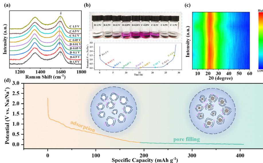
Fig. 6 (a) *Ex situ* Raman spectra (b) the corresponding color alteration of ethanol containing 1 wt% phenolphthalein after reaction with the ZHCS6-13 electrode at various potentials. (c) *Ex situ* XRD test of ZHCS6-13 electrode at selected potentials. (d) Schematic diagram of the sodium ions storage stages for ZHCS6-13.
