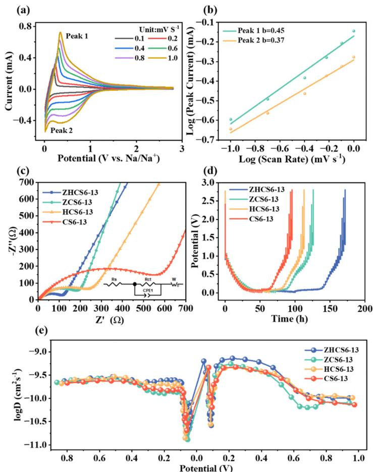
Fig. 5 (a) CV curves of ZHCS6-13 at various scanning rates from 0.1 to 1  $\text{mV s}^{-1}$  and (b) the corresponding correlations between peak current ( $i$ ) and scan rate ( $v$ ) at peak 1 and peak 2. (c) Nyquist plots, and the inset is an equivalent electrical circuit model. (d) GITT curves of samples. (e) Sodium ions diffusion coefficients during the sodiation and desodiation process.
