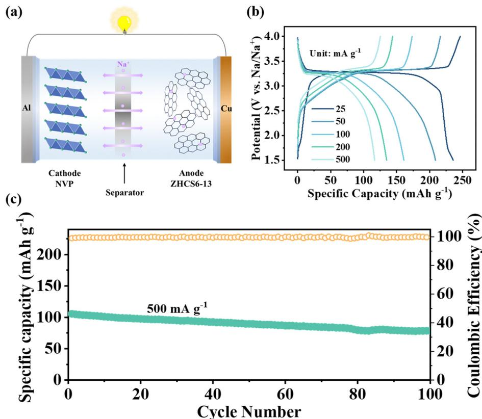
Fig. 7 Electrochemical properties of ZHCS6-13//NVP sodium-ion full cells. (a) Schematic illustration. (b) GCD curves at different current rates. (c) Cycling stability at 500 mA g<sup>-1</sup> of ZHCS6-13//NVP sodium-ion full cells.
