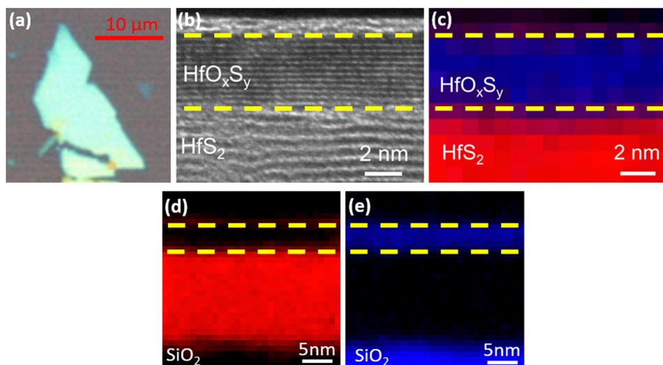
**Fig. 1** (a) Optical microscopy image of HfO<sub>x</sub>S<sub>y</sub>/HfS<sub>2</sub> flakes before being transferred to lamella for transmission electron microscopy (TEM). (b) Cross-sectional TEM image of partially oxidised flake shows crystallinity of the resulting oxide layer and (c) electron energy-loss spectroscopy (EELS) mapping of (d) sulfur (red) and (e) oxygen (blue) demonstrates a clear separation of the HfO<sub>x</sub>S<sub>y</sub> and HfS<sub>2</sub> regions.
