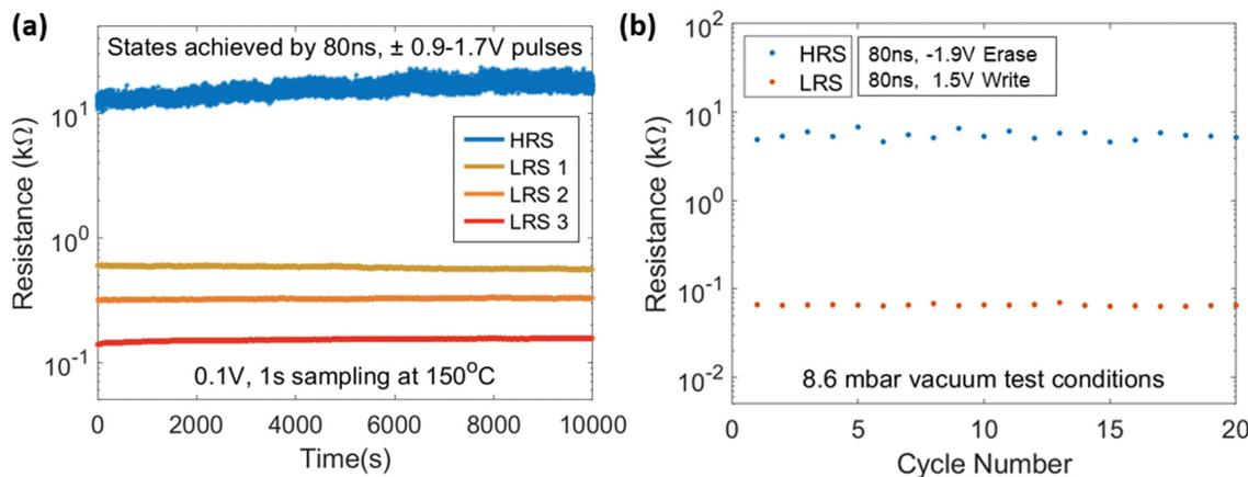
Fig. 3 (a) Non-volatile states achieved by 80 ns pulse programming are retained over  $10^4$  s at 150 °C. (b) Pulsed voltage resistance switching unaffected by operating device in an 8.6 mbar vacuum environment.
