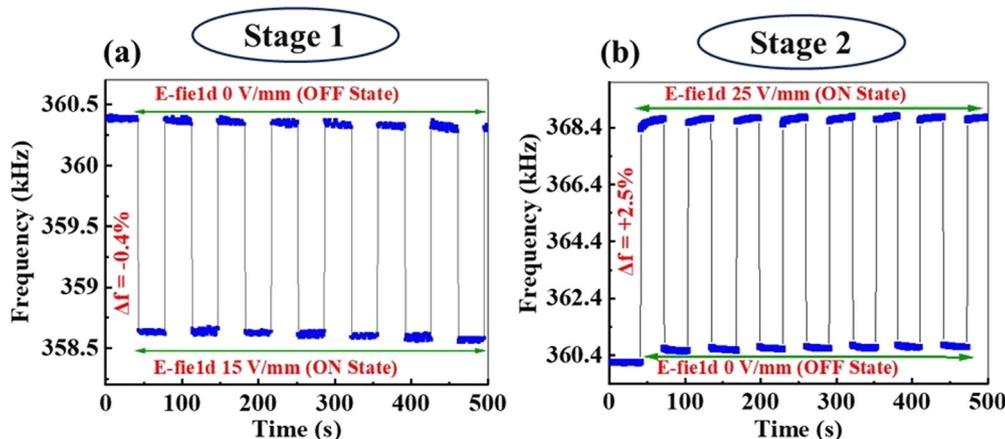
Fig. 5 Mechanical frequency modulation of the VO<sub>2</sub>/TiO<sub>2</sub> microstring as a function of time (a) at 15 V mm<sup>-1</sup> and (b) at 25 V mm<sup>-1</sup> pulsating  $E$ -field.
