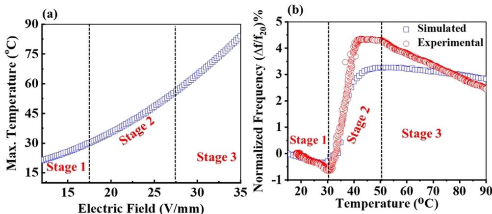
Fig. 8 (a) Maximum temperature across microstring due to applied electric field, (b) fundamental frequency variation of microstring as a function of temperature.
