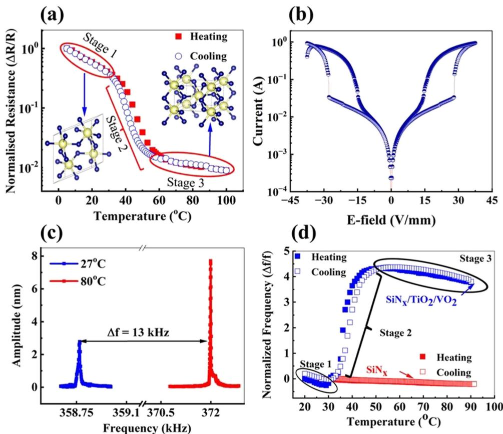
Fig. 4 (a) Resistance changes of VO<sub>2</sub> microstringing as a function of temperature. (b) Current flow in VO<sub>2</sub> microstringing when an electric-field sweep is performed across it showing E-MIT at room temperature (30 °C). (c) Amplitude response and frequency response at room temperature and high temperature (d) normalized frequency change as a function of temperature of VO<sub>2</sub>-coated and bare (SiN<sub>x</sub>) microstrings.
