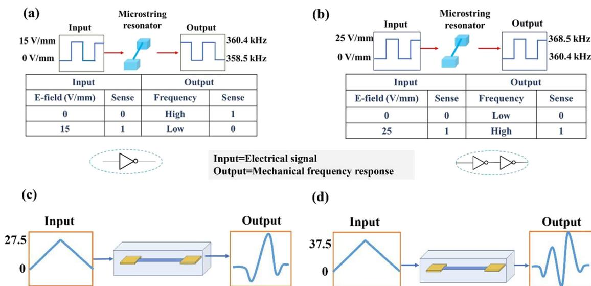
Fig. 7 Schematic sketch and truth table corresponding to (a) NOT gate, (b) buffer gate and frequency response pattern corresponding to the ramping signal from (c) 0 to  $27.5 \text{ V mm}^{-1}$ , (d) 0 to  $37.5 \text{ V mm}^{-1}$ .
