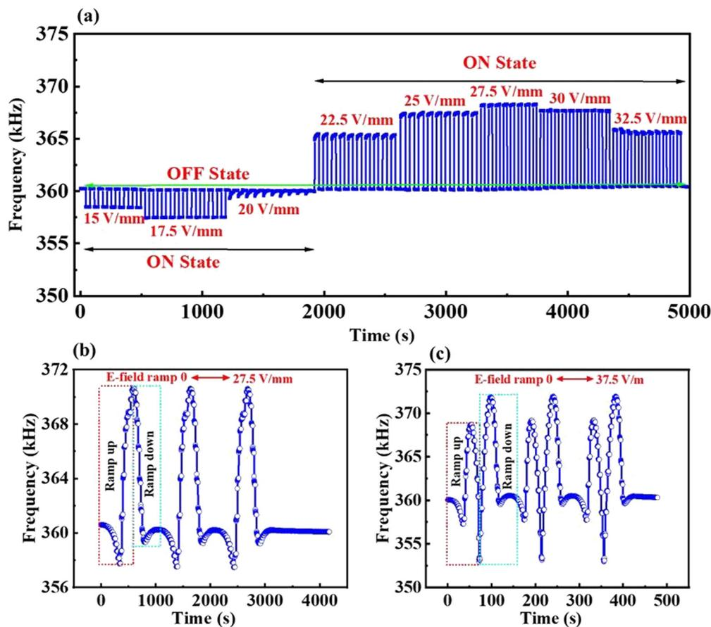
Fig. 6 (a) Frequency response of the VO<sub>2</sub> microstringing as a function of pulsating  $E$ -field from 15 V mm<sup>-1</sup> to 32.5 V mm<sup>-1</sup>, (b) and (c) frequency responses of suspended VO<sub>2</sub> microstringing as a result of ramping  $E$ -field from 0–27.5 V mm<sup>-1</sup> and 0–37.5 V mm<sup>-1</sup>.
