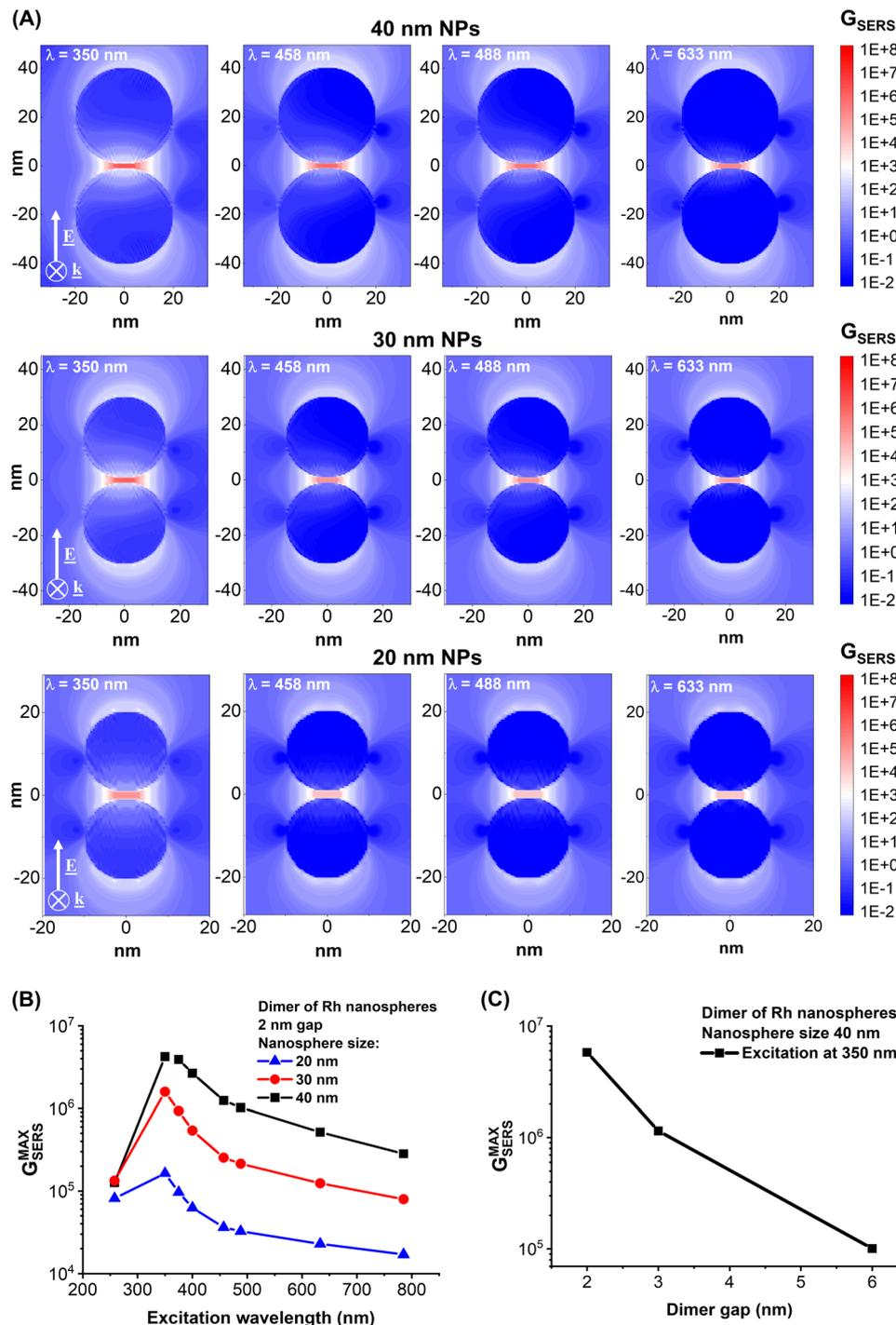
Fig. 6 (A) Bidimensional maps of the  $G_{\text{SERS}}$  in the equatorial plane of Rh NP dimers with a gap of 2 nm and sizes of 20, 30 and 40 nm excited at 350, 458, 488 and 633 nm in a medium with refractive index  $n = 1.334$ . (B) Plot of the  $G_{\text{SERS}}$  maximum versus the excitation wavelength for the three dimer sizes considered. (C) The plot of the  $G_{\text{SERS}}$  maximum versus the gap size for an excitation wavelength of 350 nm and dimers with a size of 40 nm.
