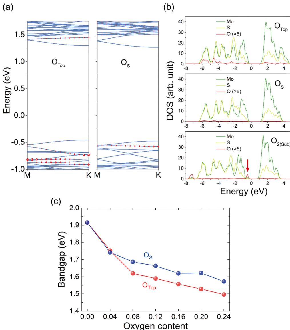
**Fig. 3** Electronic structures in oxygen-decorated  $MoS_2$ . (a) Oxygen contribution projected band structure of  $O_{Top}$  and  $O_S$ . The size of the red circle markers indicates the contribution from oxygen orbitals. (b) Partial density of states (PDOS) of  $O_{Top}$ ,  $O_S$ , and  $O_{2(Sub)}$ . The red arrow denotes the in-gap states in  $O_{2(Sub)}$ . (c) Bandgap as a function of oxygen content.
