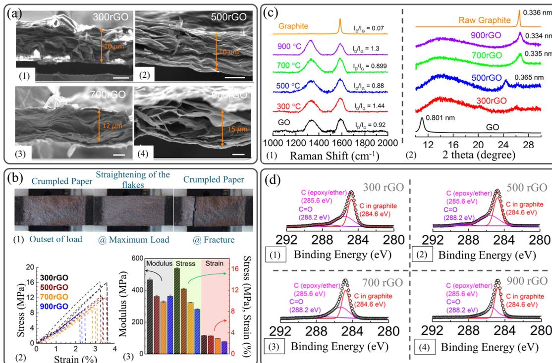
**Fig. 11** (a) SEM images showing the effect of preparation temperature on the thickness of rGO films. (b) Mechanical properties of rGO films prepared at various temperatures. (c) Raman spectra and XRD patterns of rGO prepared at various temperatures. (d) XPS of rGO prepared at different temperatures. Reproduced with permission.<sup>112</sup> Copyright © 2014, American Chemical Society.
