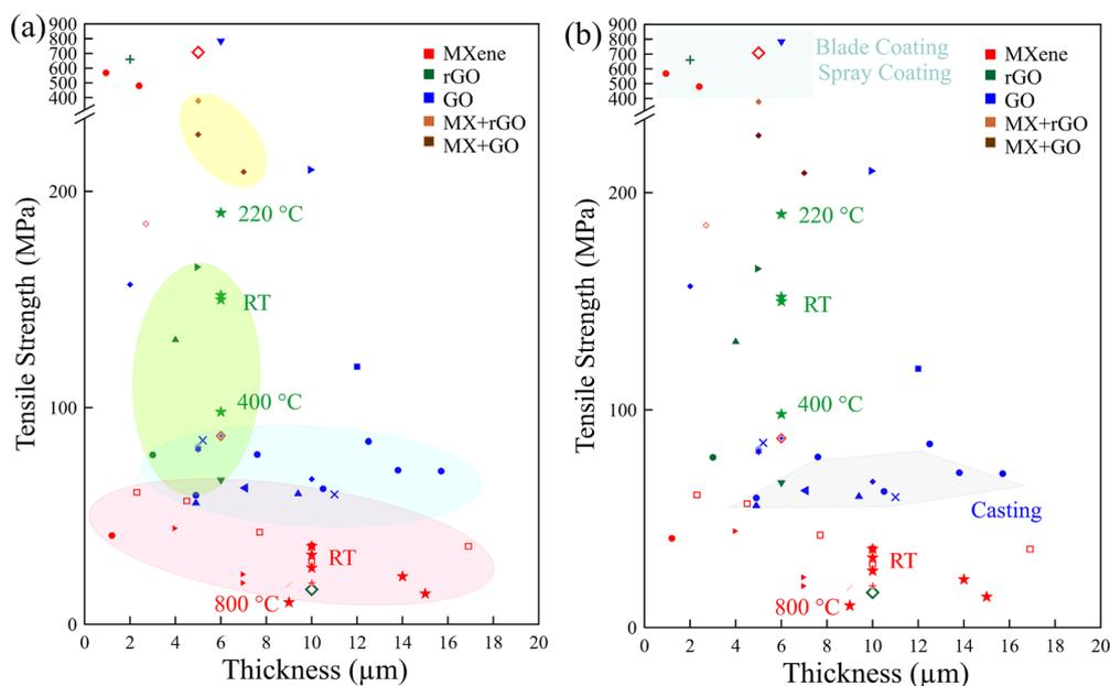
Fig. 8 Summary of (a) film thickness-dependent mechanical properties. (b) Fabrication technique-dependent mechanical properties. Most of the data were obtained at room temperature (RT); some were obtained at increased temperature, annotated in the figure. The data shown in this figure are presented in Table 2.
