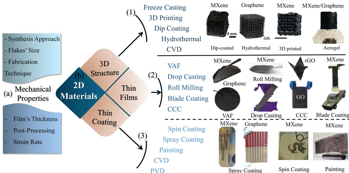
Fig. 3 (a) Factors affecting the mechanical properties of 2D material films. (b) Fabrication techniques of various 2D material structures: (1) 3D structures,<sup>150–153</sup> (2) thin films,<sup>32,42,106,125,143,154</sup> and (3) thin coatings.<sup>155–158</sup>
