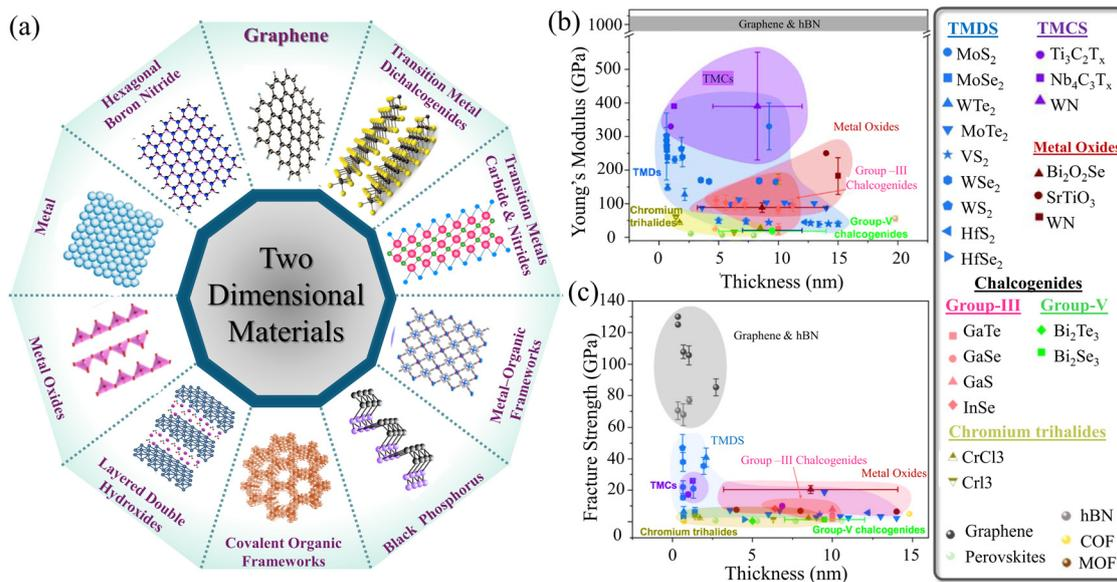
Fig. 1 (a) Schematic of different types of typical 2D nanomaterials.<sup>48,53,55,57–61,67</sup> (b) In-plane Young's modulus, and (c) in-plane fracture strength of various 2D materials. Reproduced with permission.<sup>70</sup> Copyrights © 2023, IOPSCIENCE.
