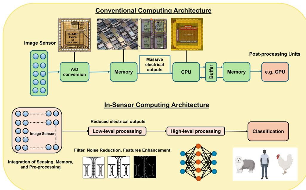
Fig. 2 Block diagrams depict the comparison between conventional imaging sensor architecture and in-sensor computing technology. Reproduced under the terms of Creative Commons CC BY License.<sup>29</sup> Copyright 2017, The Author(s), published by Springer Nature. Reproduced under the terms of Creative Commons CC BY License.<sup>30</sup> Copyright 2018, The Author(s), published by Springer Nature. Reproduced with permission.<sup>31</sup> Copyright 2021 John Wiley & Sons, Ltd.
