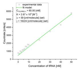
Fig. 3 Equilibrium constant determination of YO-PRO-1-tRNA complex formation (in vitro experiments). The dotted line corresponds to the fit of eqn (6).  $C_{YO-PRO-1}$  is a fitted value of initial dye concentration, K stands for the equilibrium constant,  $\alpha$  is the molecular brightness for a free dye, and  $\gamma$  – the molecular brightness of the formed complex.
