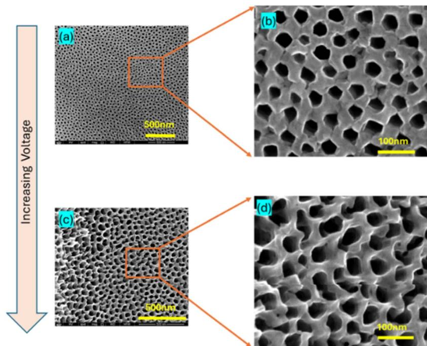
Fig. 3 SEM images of anodized Ti at varying anodization voltages in 0.1 M  $\text{NH}_4\text{F}$  + 0.1 M  $\text{H}_2\text{O}$  in ethylene glycol. (a and b) At 70 V, showing well-ordered pores; (c and d) at 80 V, showing pore wall thinning and localized dissolution effects. Images are presented at low (a and c) and high (b and d) magnifications.
