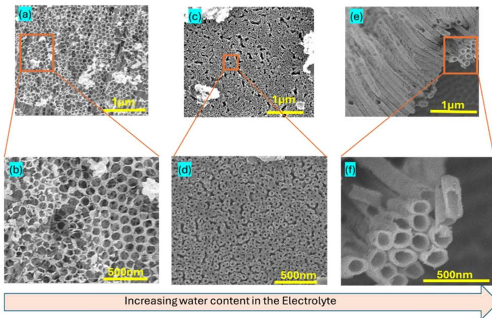
Fig. 2 SEM images of anodized Ti at different water contents in the electrolyte (0.1 M  $\text{NH}_4\text{F}$  in ethylene glycol, 70 V, and 15 min). Low- and high-magnification images illustrate the morphological transition from pores to tubes: (a and b) 0.05 M  $\text{H}_2\text{O}$ , (c and d) 0.1 M  $\text{H}_2\text{O}$ , and (e and f) 0.2 M  $\text{H}_2\text{O}$ . Uniform pore diameters of 60–70 nm were obtained at 0.1 M  $\text{H}_2\text{O}$ .
