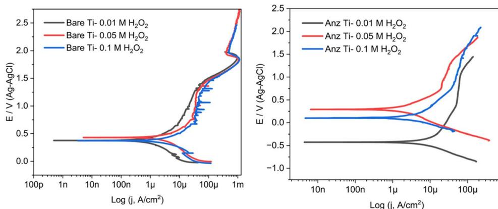
Fig. 7 Potentiodynamic polarization curves of bare and anodized Ti samples in 25 mM Na<sub>2</sub>SO<sub>4</sub> with increasing amount of H<sub>2</sub>O<sub>2</sub>. Anodized Ti shows significantly lower corrosion current densities ( $I_{\text{corr}}$ ) and more stable passive regions than bare Ti. The anodic and cathodic Tafel slopes highlight improved barrier properties of the anodized oxide, particularly after annealing, under oxidizing conditions.
