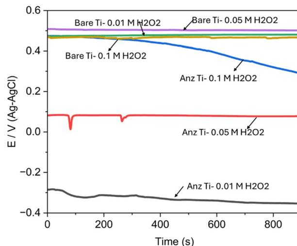
Fig. 6 Open circuit potential (OCP) evolution of bare and anodized Ti samples in 25 mM  $\text{Na}_2\text{SO}_4$  with increasing  $\text{H}_2\text{O}_2$  concentrations (0–0.1 M). Bare Ti shows relatively stable OCP values with slight negative shifts at higher peroxide contents. At the same time, anodized Ti initially exhibits more negative OCP but progressively shifts to positive potentials at higher  $\text{H}_2\text{O}_2$ , indicating adaptive passivation of the anodic oxide layer.
