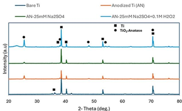
Fig. 4 XRD diffraction patterns of bare Ti, anodized Ti, and anodized Ti after corrosion studies in 25 mM  $\text{Na}_2\text{SO}_4$  without and with 0.01 M  $\text{H}_2\text{O}_2$ . The anatase  $\text{TiO}_2$  phase is visible after anodization and becomes more prominent after corrosion in oxidizing environments, demonstrating structural stability and enhanced oxide crystallinity.
