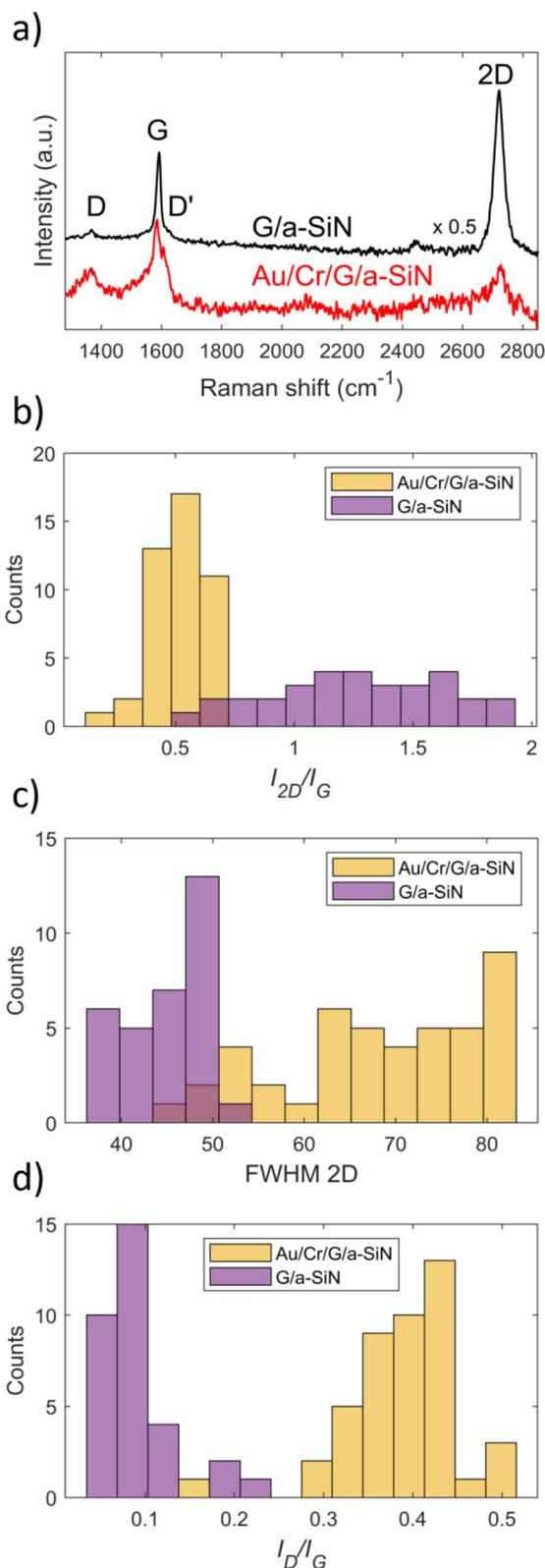
**Fig. 2** (a) Representative Raman spectra of graphene with (Au/Cr/G/a-SiN curve) and without (G/a-SiN curve) metallic contact; histograms of (b)  $I_{2D}/I_G$ , (c) FWHM of 2D and (d)  $I_D/I_G$  for Au/Cr/G/a-SiN vs. G/a-SiN.
