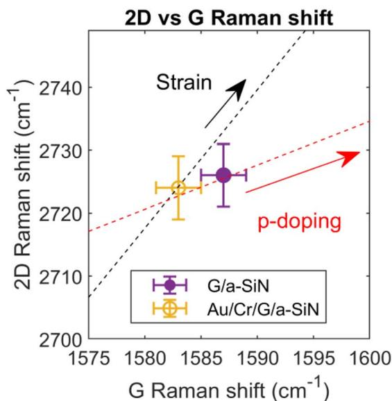
Fig. 4 Correlation analysis of 2D-G positions on G/a-SiN and Au/Cr/G/a-SiN. The dotted red line represents the direction of doping (slope 0.7), while the black dotted line represents the strain (slope 2.2).
