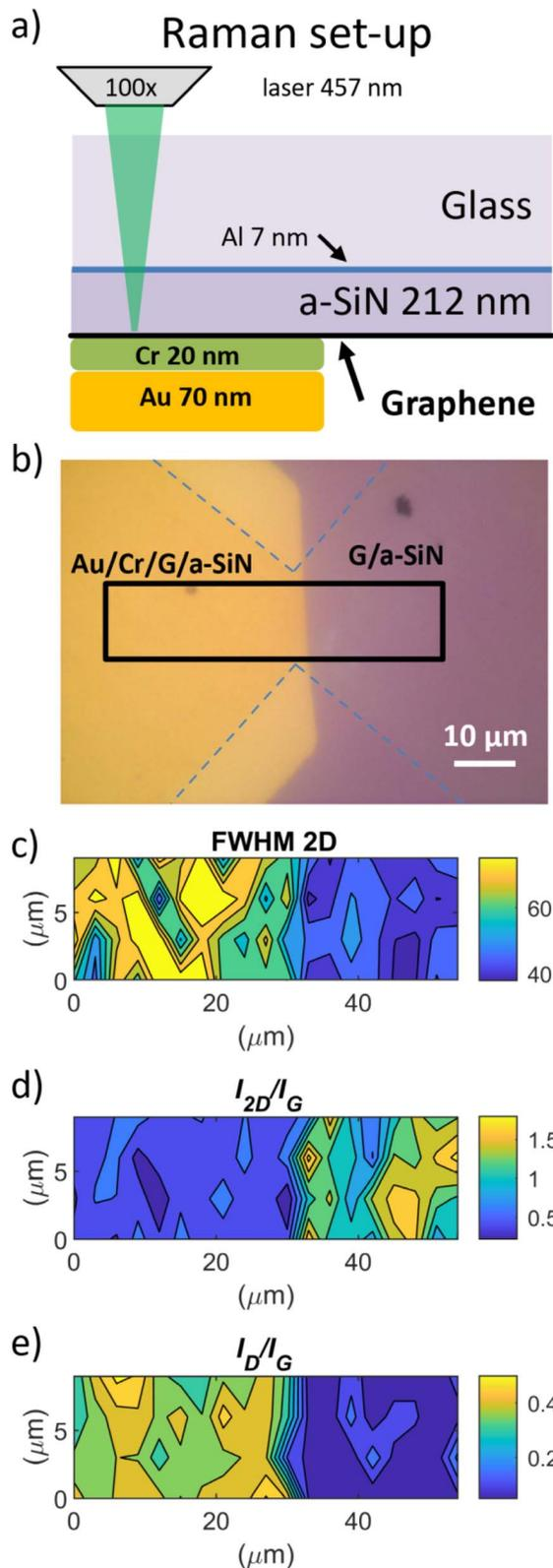
**Fig. 3** (a) Scheme of the Raman measurement set-up for graphene on a transparent substrate in upside down configuration. (b) Micrograph of the VdP test structure with graphene under metallic contact (Au/Cr/G/a-SiN) at left and graphene without metallic contact (G/a-SiN) at right; the black rectangle represents the area of the sample probed by micro Raman. Raman maps of intensities of (c) FWHM for 2D signal, (d)  $I_{2D}/I_G$  and (e)  $I_D/I_G$ .
