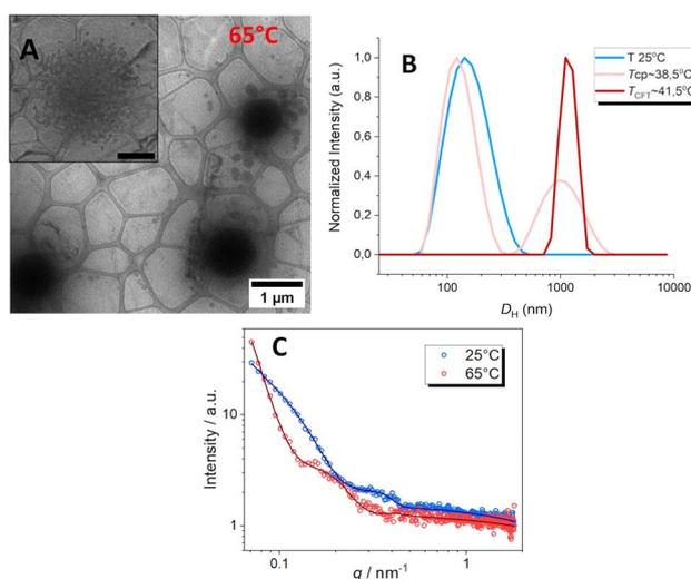
Fig. 5 (A) Representative cryo-TEM image of PTEGMA<sub>78</sub>-*b*-PDPA<sub>85</sub> (entry 6) nano-objects at 65 °C. The scale bars in the zoomed cryo-TEM image represent 1  $\mu\text{m}$ ; (B) DLS plot for the  $D_{\text{H}}$  at  $T = 25$  °C (blue curve),  $T_{\text{cp}}$  38.5 °C (light pink curve) and at the  $T_{\text{CFT}} = 41.5$  °C (see the dark red curve); (C) SAXS profile at 25 °C (in blue) and 65 °C (in red).
