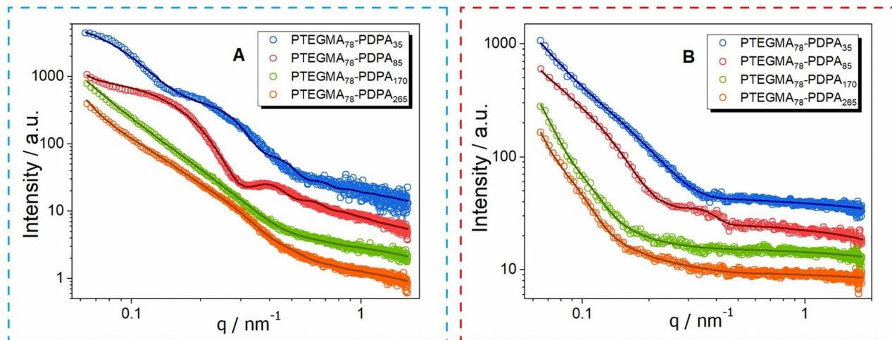
Fig. 3 Fitted SAXS curves of PTEGMA<sub>78</sub>-*b*-PDPA<sub>*n*</sub> prepared via aqueous emulsion RAFT/PISA at (A) 45 °C or (B) 70 °C.
