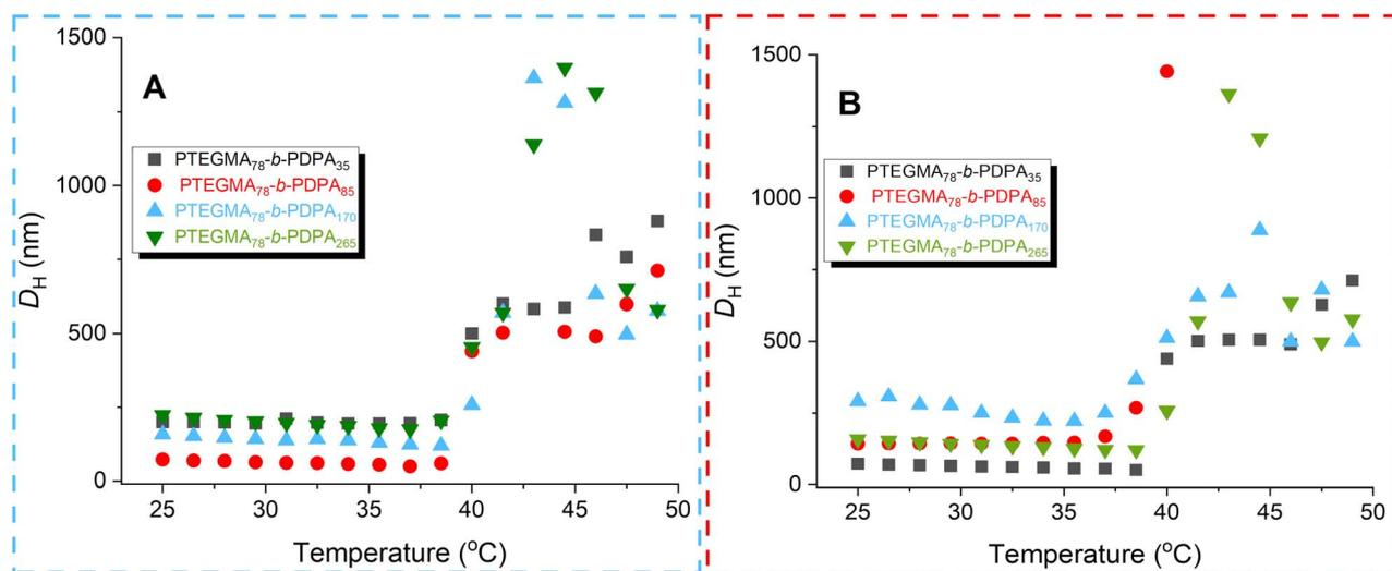
Fig. 4 Temperature dependence of the  $D_H$  of PTEGMA<sub>78</sub>-*b*-PDPA<sub>*n*</sub> nano-objects: (A) entries 1–4 and (B) entries 5–8 (Table 2).
