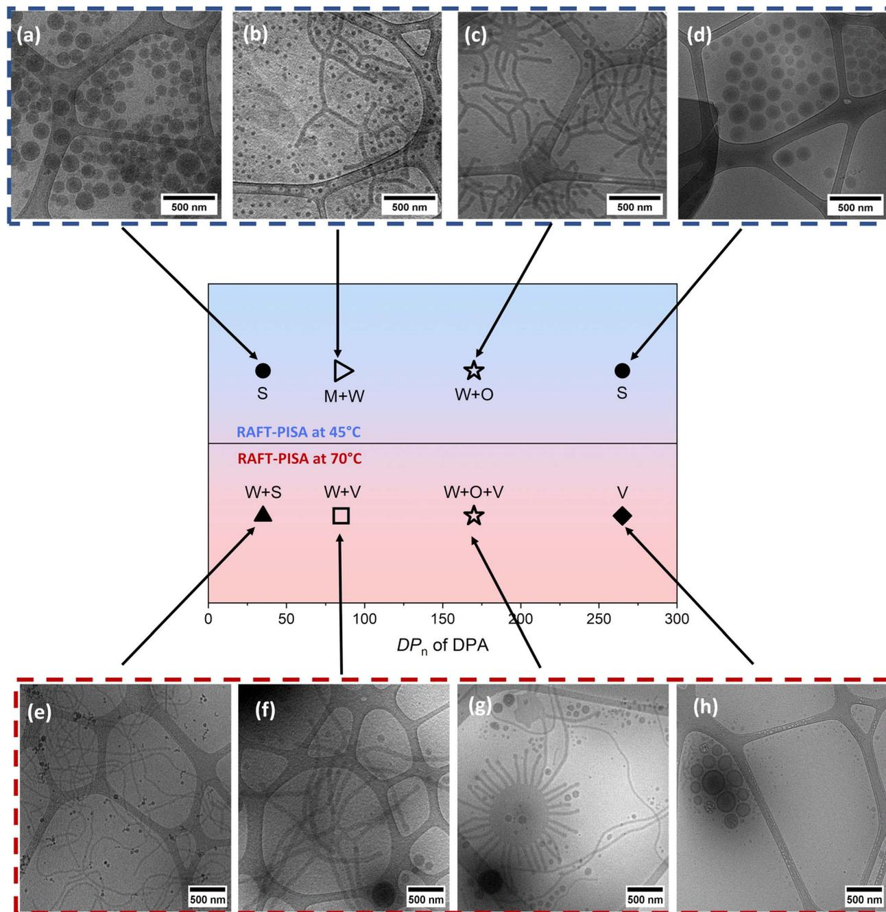
Fig. 2 Phase diagram of NPs prepared with varying target  $DP_n$  of the hydrophobic core-forming block via aqueous RAFT emulsion polymerization at 45 °C (cryo-TEM images (a)–(d); entries 1–4, in Table 1) and 70 °C (cryo-TEM images (e)–(h); entries 5–8, in Table 1), conducted at 10 wt% solids, along with the corresponding cryo-TEM images. Keys: S = spheres, W + S = worms + spheres, W + O + V = worms + “octopus” + vesicles, V = vesicles, M + W = micelles + worms, and W + V = worms + vesicles.
