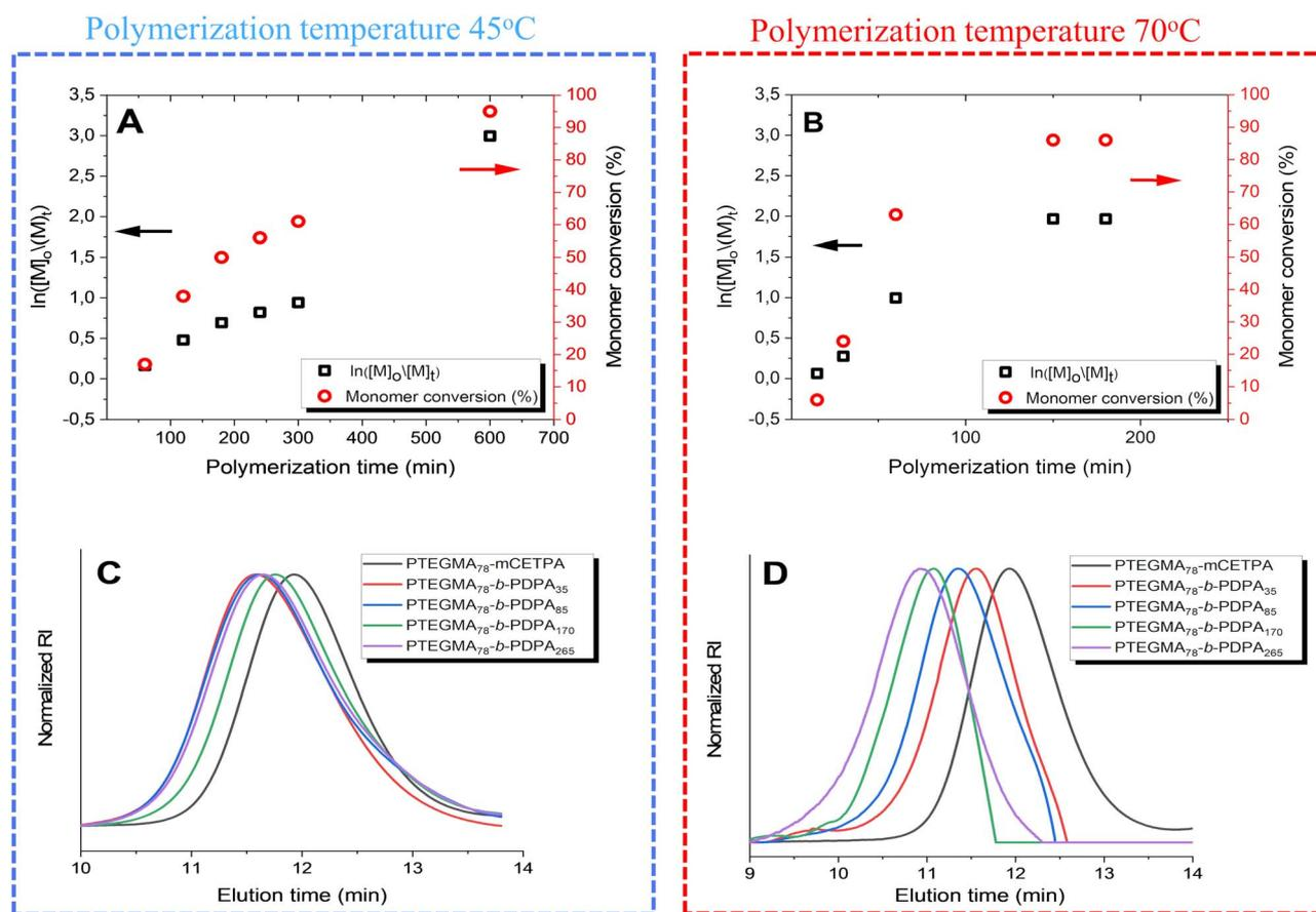
Fig. 1 Monomer conversion vs. time profiles (red circles) alongside semi-logarithmic plots (black squares) for PTEGMA<sub>78</sub>-b-PDPA<sub>265</sub> NPs polymerized at 45 °C (A) and 70 °C (B). Normalized SEC traces of the PTEGMA<sub>78</sub>-mCETPA (black curve) and the corresponding PTEGMA<sub>78</sub>-b-PDPA<sub>n</sub> NPs obtained at 45 °C (C) and 70 °C (D), respectively. All SEC analyses were performed in DMF containing LiBr (1 g L<sup>-1</sup>) (see Table 1).
