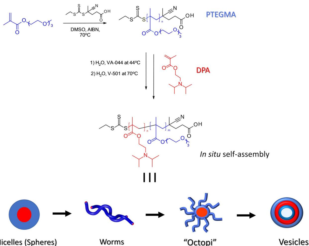
**Scheme 1** Schematic overview of the aqueous emulsion RAFT/PISA process for fabricating dual thermo- and pH-responsive PTEGMA-*b*-PDPA diblock copolymer nanoassemblies at polymerization temperatures of 45 °C and 70 °C.
