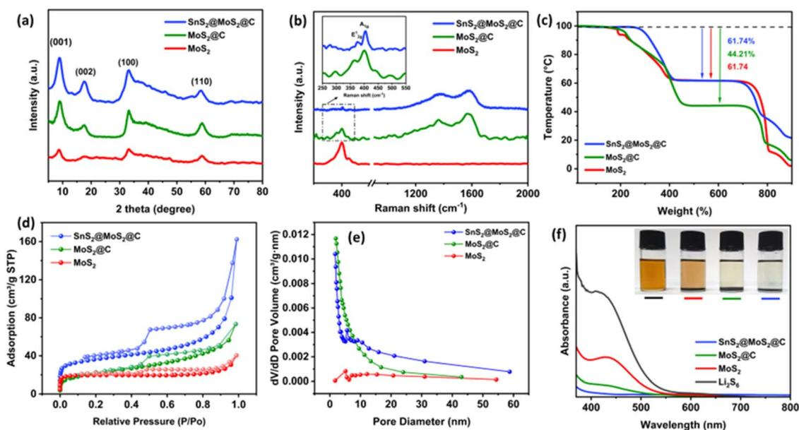
Fig. 2 (a) XRD patterns, (b) Raman spectra, (c) nitrogen adsorption–desorption isotherms, (d) corresponding pore size distribution, (e) TGA curve and (f) UV-vis absorption spectra of  $\text{Li}_2\text{S}_6$  solution (the inset shows the visualized adsorption in  $\text{Li}_2\text{S}_6$  solution after standing for four hours) of  $\text{SnS}_2@MoS_2@C$ ,  $MoS_2@C$ , and  $MoS_2$ .
