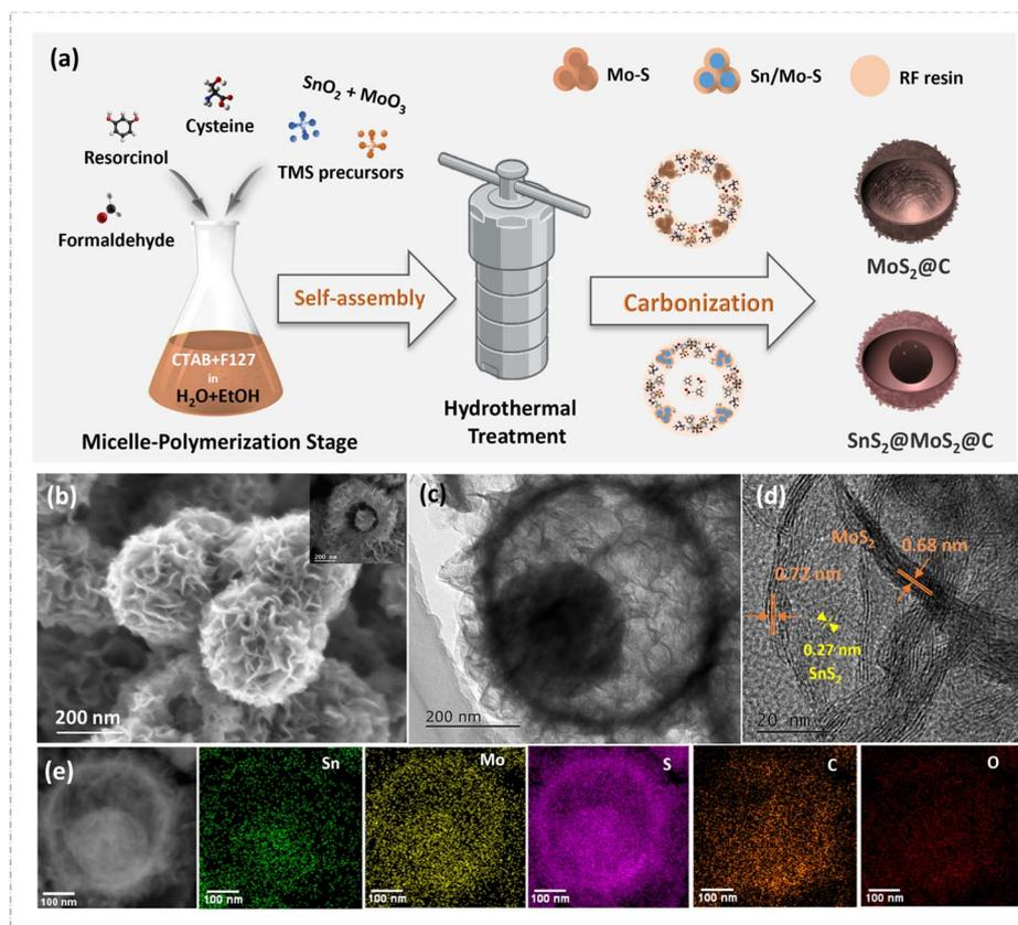
Fig. 1 (a) Schematic illustration of the synthesis and the possible mechanism of the formation of spherical  $\text{SnS}_2@\text{MoS}_2@\text{C}$  yolk-shell nanospheres through a one-pot self-assembly process. (b) SEM image and (c) TEM image. (d) HRTEM image showing 1T/2H- $\text{MoS}_2$  lattice fringes and  $\text{SnS}_2$  planes and (e) TEM dark field and EDS-mapping of Sn, Mo, S, C, and O.
