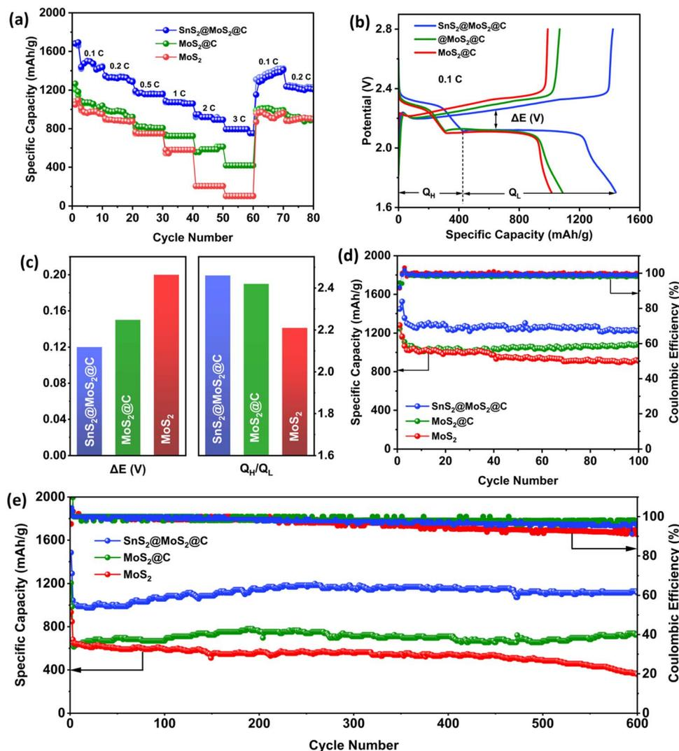
Fig. 5 (a) Rate performance, (b) discharging–charging profiles at 0.1C, (c) overpotentials ( $\Delta E$ ) and phase conversion coefficient ( $Q_H/Q_L$ ) profiles, (d) cycling stability and coulombic efficiency at 0.2C after 100 cycles, and (e) long-term cycling stability and coulombic efficiency at 1C of  $\text{SnS}_2@MoS_2@C$ ,  $MoS_2@C$  and  $MoS_2$  Li–S batteries.
