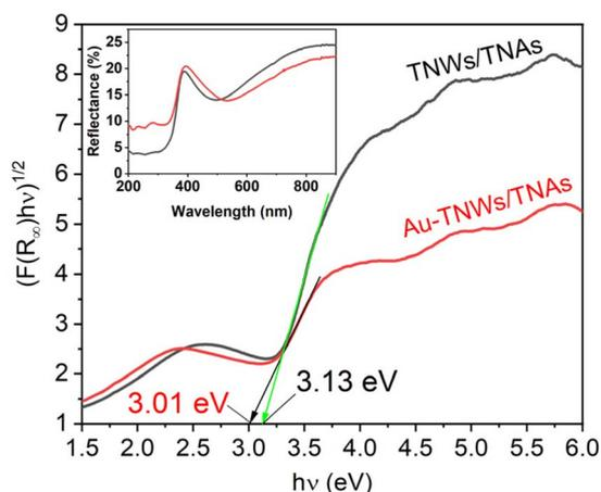
Fig. 9 Tauc plots derived from the transformed Kubelka–Munk function  $[F(R_{\infty}) \cdot h\nu]^{0.5}$  as a function of photon energy, used to estimate the optical band gaps of TNWs/TNAs and Au-TNWs/TNAs. The extrapolated linear regions indicate the corresponding band gap energies. The inset shows the diffuse reflectance spectra (DRS) of both samples.
