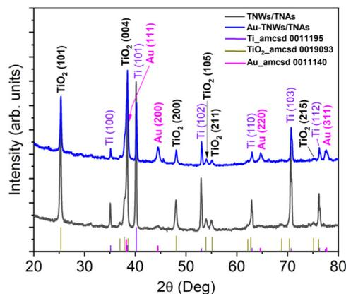
Fig. 1 XRD patterns of TNWs/TNAs and Au-decorated TNWs/TNAs. Reference powder XRD patterns from the AMCSD database for Ti, anatase-phase TiO<sub>2</sub>, and Au are included in the figure for comparison.
