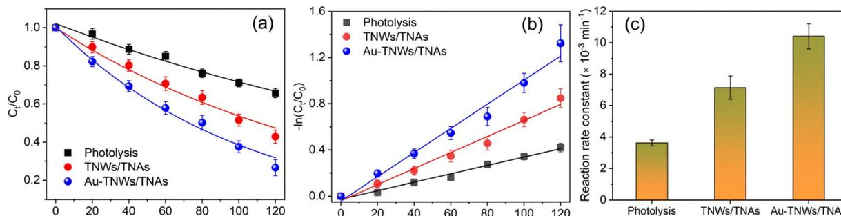
Fig. 6 (a) Photodegradation kinetics of methylene blue (MB) under UV-vis irradiation via photolysis and photocatalysis using TNWs/TNAs and Au-TNWs/TNAs. (b) Corresponding  $-\ln(C_t/C_0)$  vs. time plot derived from the data in (a). (c) Reaction rate constants ( $k$ ) for MB degradation under photolytic and photocatalytic conditions using TNWs/TNAs and Au-TNWs/TNAs.
