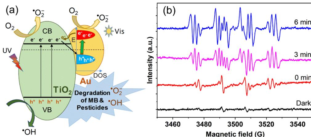
Fig. 10 (a) Proposed mechanism for the photocatalytic degradation of methylene blue (MB) and pesticides by Au-TiO<sub>2</sub> under UV-vis illumination. (b) DMPO-•OH radical EPR spectrum for Au-TNWs/TNAs.
