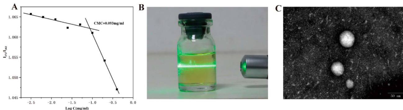
Fig. 1 Self-assembled amphiphilic chitosan-curcumin (ACS-Cur) nanomicelles; (A) critical micelle concentration determination via pyrene fluorescence; (B) Tyndall effect in ACS-Cur suspension indicating nanomicelle formation; (C) TEM image showing spherical morphology (scale bar = 50 nm). (Note: Reproduced from ref. 36, Molecules , 29, 2693 (CC BY 4.0).)
