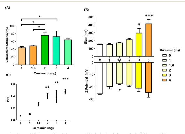
Fig. 4 Curcumin entrapment efficiency and its effect on nanoparticle physicochemical properties in PLGA nanoparticles prepared *via* nanoprecipitation: (A) entrapment efficiency (% EE) of curcumin at different loading concentrations (B) influence of curcumin loading on particle size and zeta potential. (C) Effect on polydispersity index (Pdi) at varying curcumin loads. (*Note*: Reproduced from ref. 67, *Pharmaceutics*, **15**, 1594. CC BY 4.0.)
