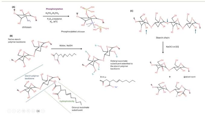
Fig. 6 Diversification of biopolymers by (A) phosphorylation,<sup>83</sup> (B) esterification,<sup>84</sup> (C) oxidation.<sup>85</sup>
