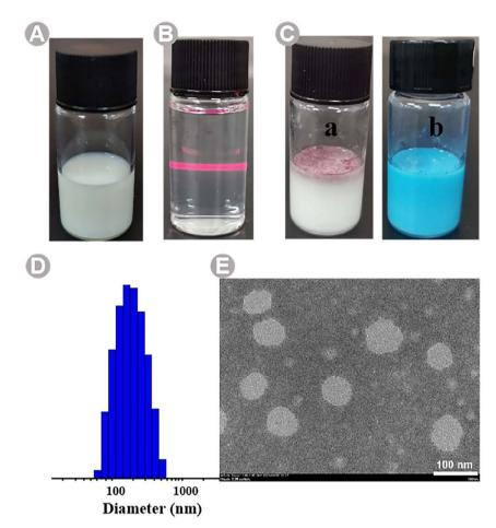
Fig. 3 Physicochemical characterization of BB-TTO nanoemulsions (NEs): (A) appearance and shape; (B) Faraday–Tyndall effect after dilution; (C) oil-in-water type identification using (a) Sudan red and (b) methylene blue; (D) particle size distribution (~160 nm); (E) TEM image showing spherical, smooth, well-dispersed droplets. (*Note*: Reproduced from ref. 58, *Molecules*, 28, 5889, licensed under CC BY 4.0.)
