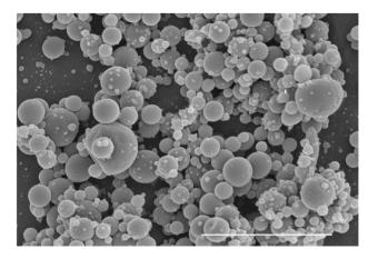
Fig. 5 SEM image of electrosprayed agar nanocapsules loaded with 5 wt% chlorophyllin sodium copper salt (CHL) relative to agar content. Scale bar: 4 µm. (Note: Reproduced from ref. 76, Foods, 11, 2093. CC BY 4.0.)
