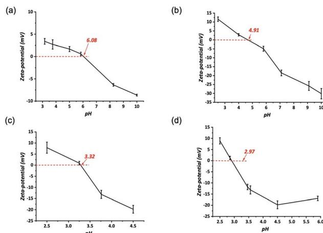
Fig. 5 Zeta potential of different types of leather. (a) Raw goat skin; (b) TWS-tanned; (c) vegetable-tanned; and (d) vegetable-aldehyde combination tanned.
