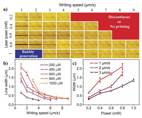
Fig. 1 (a) Microscope images of the printed lines for various laser powers and writing speeds (scale bar 10 μm), (b) plot of the line width as a function of writing speed for various laser powers, and (c) plot showing the variation of line width as a function of laser power for various writing speeds.
