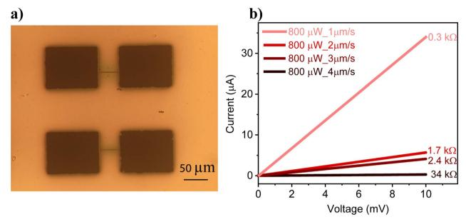
Fig. 3 (a) The printed Ag lines across a 50 μm gap electrode. (b) The I-V characteristics of Ag conducting lines printed at 800 μW power and a writing speed of 1-4 μm s<sup>-1</sup>.
