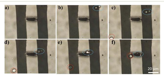
Fig. 4 (a) The printed conducting line of resistance  $\sim 1~\text{k}\Omega$  between the gap electrode and (b-f) sequences from the electrothermal trapping event of the yeast cells (at a voltage of 1 V).
