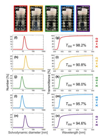
Fig. 2 Colloidal characteristics of as-synthesized  $TiO_2$ -OA/OAm in chloroform. (a)–(e) Photos, (f), (h), (j), (l) and (n) solvodynamic size distributions obtained by DLS measurement, and (g), (i), (k), (m) and (o) light transmittance obtained by UV-vis spectroscopy of colloidal solutions of  $TiO_2$  NPs in chloroform in cases of (a), (f) and (g) X=0.0, (b), (h) and (i) X=0.3, (c), (j) and (k) X=0.6, (d), (l) and (m) X=0.8, and (e), (n) and (o) X=1.0, where X=[OA]/([OA]+[OAm]).
