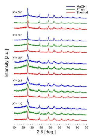
Fig. 4 XRD patterns for  $TiO_2$  NPs for comparison between three strategies of surface ligand removal: (blue line) washing with methanol, (green line) washing with  $F^-$  ions, and (red line) thermal treatment at 600 °C. X = OA/(OA) + OAM).
