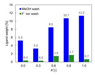
Fig. 3 Ligand weight of TiO<sub>2</sub> NPs washed with (blue) methanol and (green)  $F^-$  ions, plotted as a function of the OA/OAm ratio (X = [OA]/([OA] + [OAm])). The values were obtained by elemental analysis.
