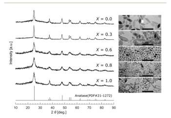
Fig. 1 XRD patterns and TEM images of synthesized  $TiO_2$  NPs. X = [OA]/([OA] + [OAm]). The scale bars are 50 nm.
