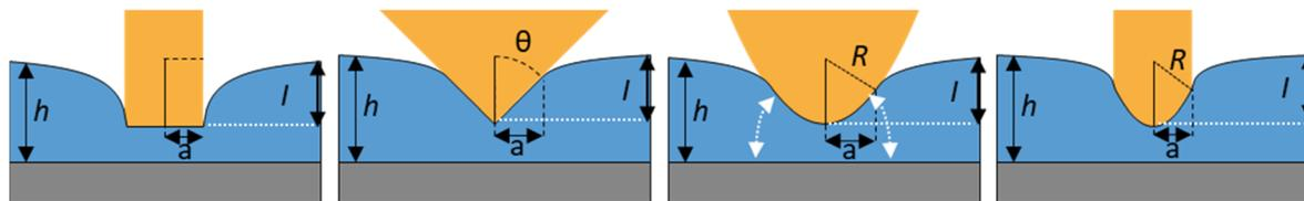
Fig. 3 Schematic diagrams of the most common axisymmetric tip geometries in AFM nanomechanical mapping. From left to right, cylinder, conical tip, paraboloid and nanowire. The sample thickness  $h$ , tip geometry parameters, indentation  $l$  and projected radius of the contact area  $a$  are illustrated. The bottom stiffness effect is schematized for a paraboloid (white arrows).
