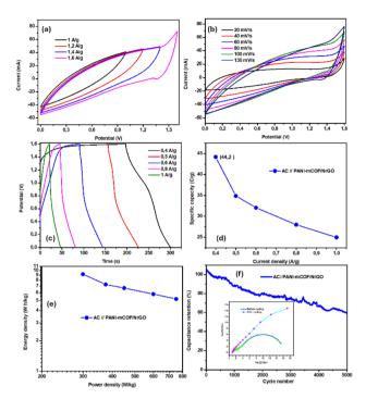
Fig. 5 (a) CV curves of the AC//PANI-COF/NrGO at various potential windows (constant 20 mV s<sup>-1</sup>), (b) CV curves of the AC//PANI-COF/NrGO at various scan rates, (c) GCD curves of the asymmetric device at various current densities, (d) specific capacity vs. current density of the device, (e) ragone plot of the AC//PANI-COF/NrGO device, and (f) cycling stability testing of the device (insert: EIS before and after cycling).
