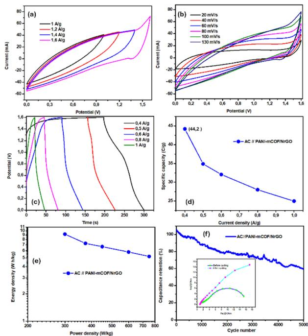
Fig. 5 (a) CV curves of the AC//PANI-COF/NrGO at various potential windows (constant  $20 \text{ mV s}^{-1}$ ), (b) CV curves of the AC//PANI-COF/NrGO at various scan rates, (c) GCD curves of the asymmetric device at various current densities, (d) specific capacity vs. current density of the device, (e) ragone plot of the AC//PANI-COF/NrGO device, and (f) cycling stability testing of the device (insert: EIS before and after cycling).
