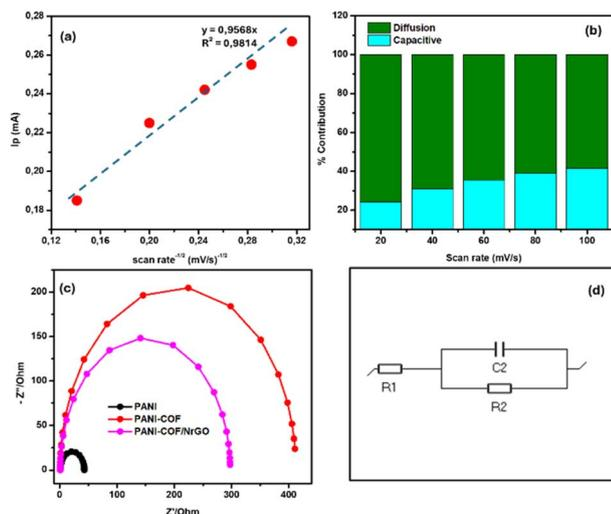
Fig. 4 (a) peak current ( $I_p$ ) vs.  $\sqrt{\text{scan rate}}$  Curve for the PANI-COF/NrGO composite, (b) percentage contributions of the diffusion and capacitive processes at different scan rates, (c) fitted EIS curves of PANI, PANI-COF, and PANI-COF/NrGO composite, (d) circuit used for fitting the EIS data.
