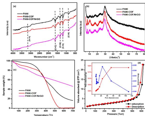
Fig. 1 (a) FTIR patterns of PANI, PANI/COF, and PANI-COF/NrGO composite, (b) XRD patterns of PANI-COF and PANI-COF/NrGO, (c) TGA spectrum of PANI, PANI-COF, and PANI-COF/NrGO, (d) N<sub>2</sub> adsorption–desorption isotherms for PANI-COF/NrGO.
