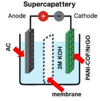
Scheme 2 Illustration of the supercapattery device
