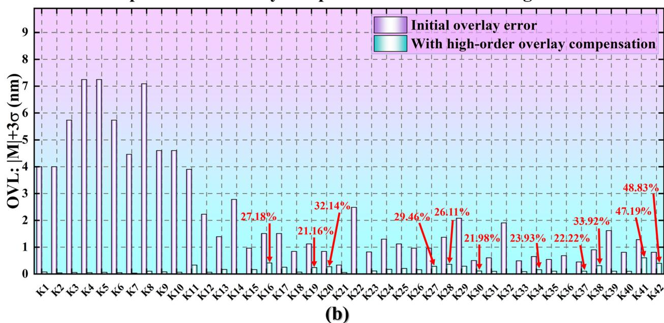
Fig. 7 Correction effect diagram of the high-order correction model under the  $k$ -parameter limit case. (a) The overlay compensation effect of the expansion effect under the  $k$ -parameter limit. (b) The overlay compensation effect of the shrinkage effect under the  $k$ -parameter limit.
