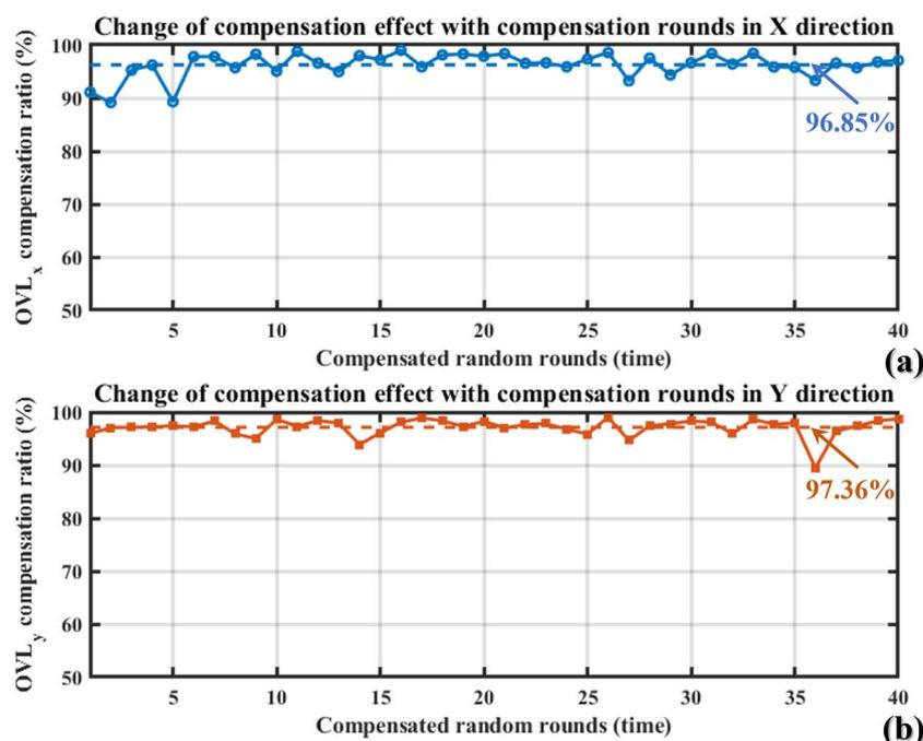
Fig. 4 The average correction effect of the overlay error. (a) The compensation effect in the  $x$ -direction after several random overlay compensations. (b) The compensation effect in the  $y$ -direction after several random overlay compensations.
