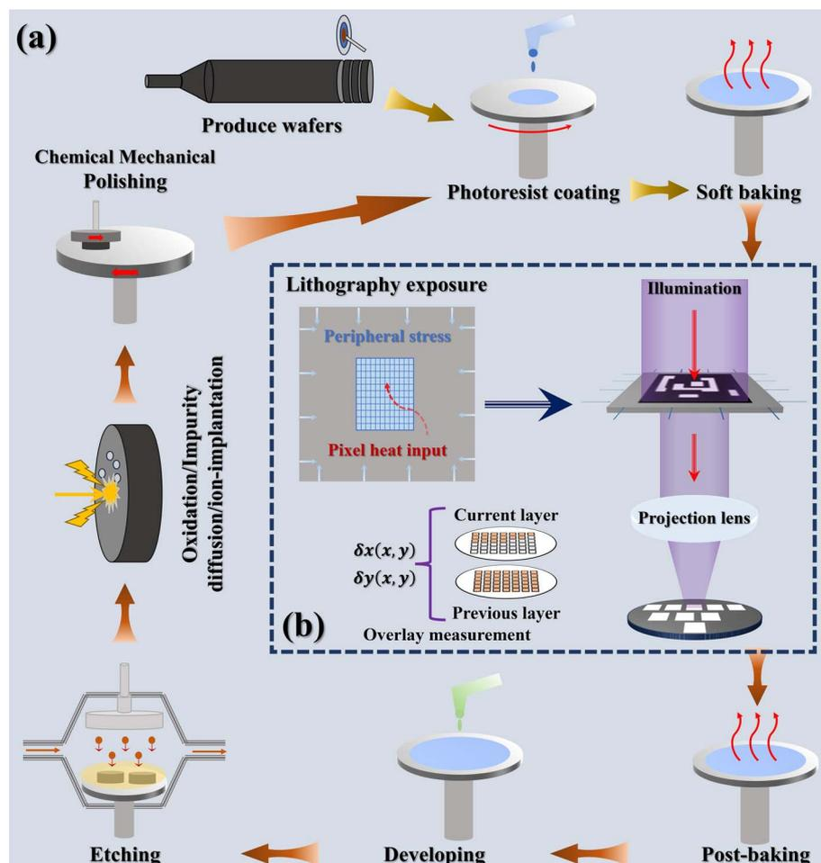
Fig. 1 Schematic diagram of the modern IC manufacturing process and the high-order overlay error correction in the advanced lithography process.<sup>19,28</sup> (a) Modern IC manufacturing process. (b) The high-order overlay error correction in the advanced lithography process.
