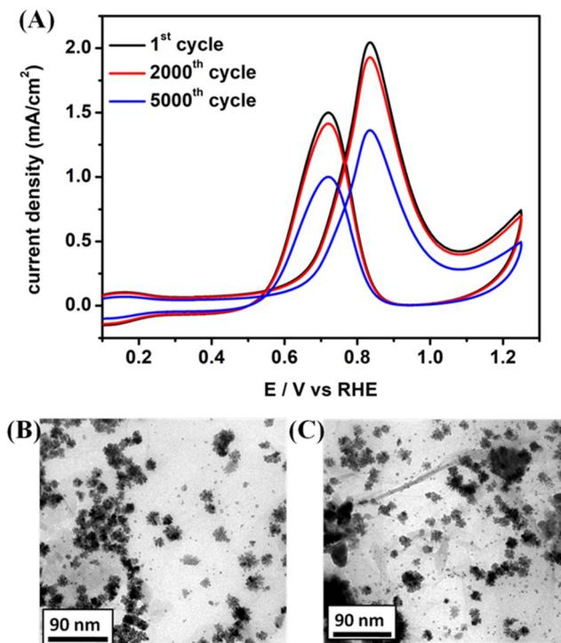
Fig. 6 (A) Accelerated durability test (ADT) for the PtPd NDs/RGO catalyst in the same environment at a scan rate of  $100 \text{ mV s}^{-1}$  for up to 2000 cycles and 5000 cycles, and morphological analysis for the PtPd NDs/RGO catalyst. (B) TEM image before ADT and (C) TEM image after ADT.
