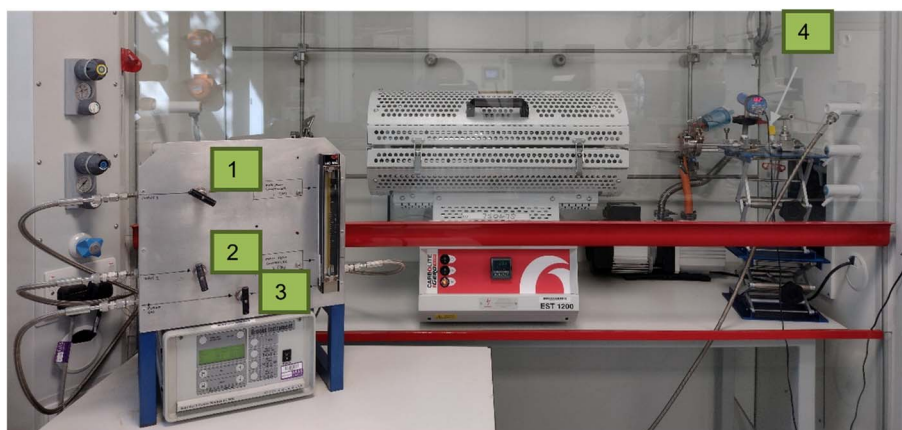
Fig. 10 CVD set up; 1 and 2 hydrogen and methane mass flow controllers, respectively, 3 rotameter for argon, and 4 the vent valve.
