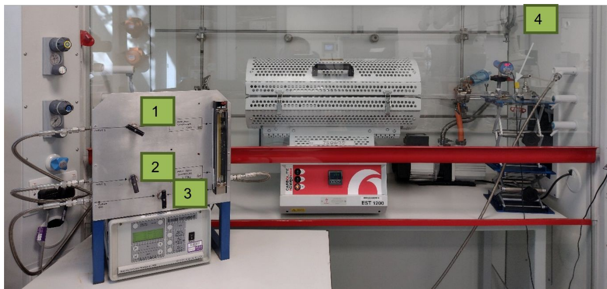
Figure 10 CVD set up; 1 and 2 hydrogen and methane mass flow controllers, respectively, 3 rotameter for argon, and 4 the vent valve.
