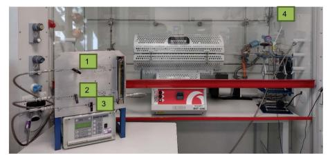
Fig. 10 CVD set up; 1 and 2 hydrogen and methane mass flow controllers, respectively, 3 rotameter for argon, and 4 the vent valve.
