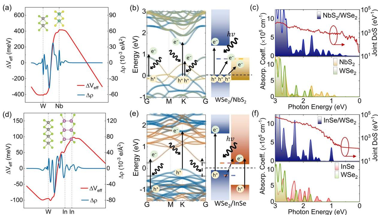
Fig. 2 (a) Effective potential variation ( $\Delta V_{\text{eff}}$ ) and charge redistribution ( $\Delta\rho$ ), (b) band structure and band diagram, and (c) absorption coefficient and joint DoS for the NbS<sub>2</sub>/WSe<sub>2</sub> vdW junctions. (d) Effective potential variation and charge redistribution, (e) band structure and band diagram, and (f) absorption coefficient and joint DoS for the InSe/WSe<sub>2</sub> vdW junctions.
