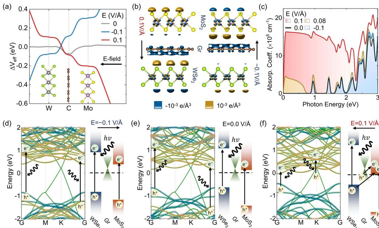
Fig. 3 (a) Effective potential variations ( $\Delta V_{\text{eff}}$ ) for the MoS<sub>2</sub>/Graphene/WSe<sub>2</sub> (MGW) junction under electric field biases. (b) Charge redistributions ( $\Delta\rho$ ) under electric field biases. (c) Absorption spectra of the MGW junction and corresponding band diagrams under electric fields of (d)  $-0.1 \text{ V } \text{\AA}^{-1}$ , (e)  $0.0 \text{ V } \text{\AA}^{-1}$ , and (f)  $+0.1 \text{ V } \text{\AA}^{-1}$ .
