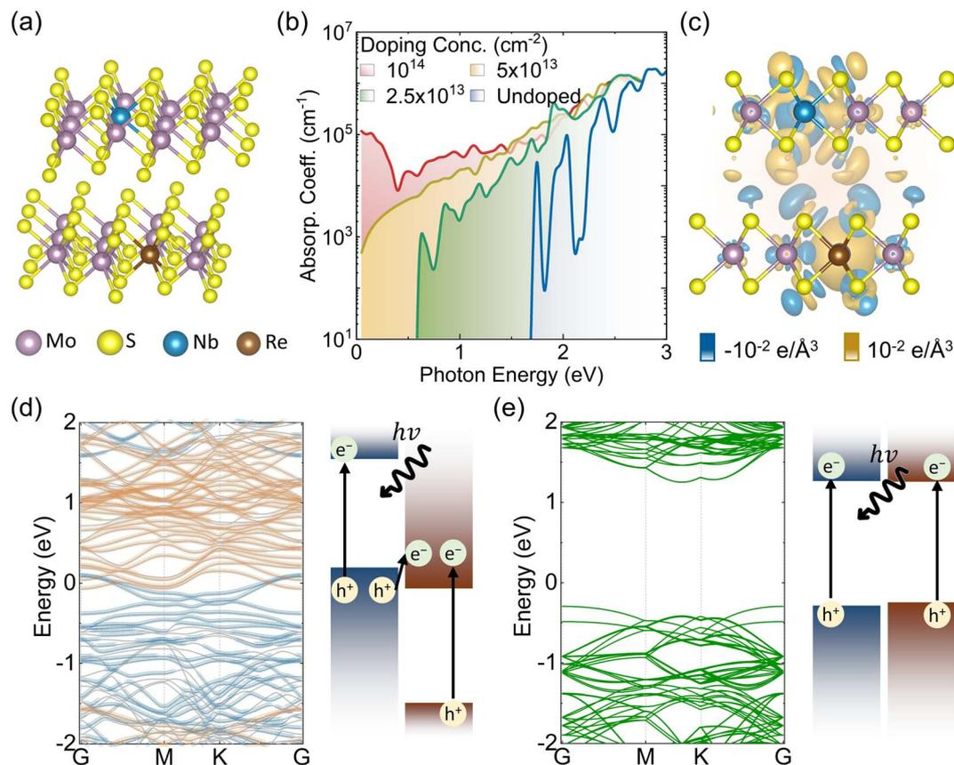
Fig. 4 (a) Atomic structure of the bilayer MoS<sub>2</sub> vdW p-n homojunction. (b) Absorption spectrum of the MoS<sub>2</sub> p-n junction. (c) Charge redistribution ( $\Delta\rho$ ) for the MoS<sub>2</sub> p-n junction compared with the intrinsic bilayer MoS<sub>2</sub>. Band structure and band diagram for (d) the bilayer MoS<sub>2</sub> p-n junction and (e) the intrinsic bilayer MoS<sub>2</sub>.
