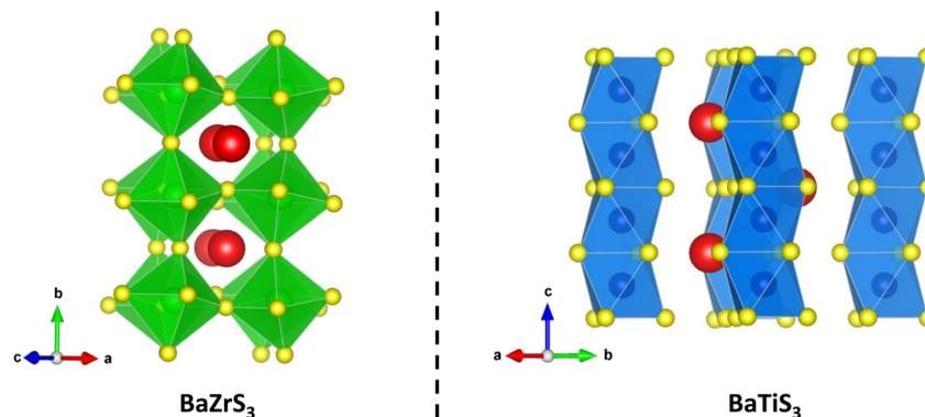
Fig. 1 The structures of  $\text{BaZrS}_3$  and  $\text{BaTiS}_3$  are shown. Ba atoms are illustrated in red, Zr atoms in green, Ti atoms in blue, and S atoms in yellow.  $\text{BaZrS}_3$  crystallizes in an orthorhombic lattice with the  $Pnma$  space group, whereas  $\text{BaTiS}_3$  is shown in a hexagonal lattice with the  $P6_3/mmc$  space group. The structures are drawn using VESTA.<sup>14</sup>
