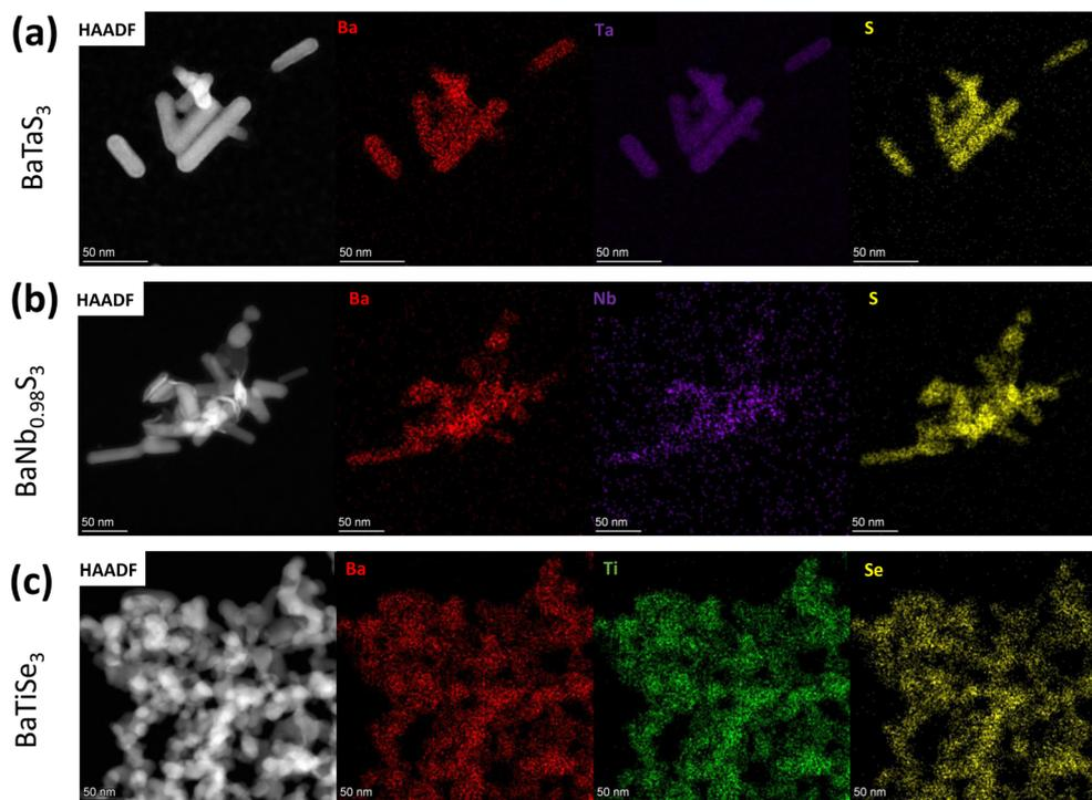
Fig. 4 STEM-EDX emission maps of the different nanocrystals showcase a uniform distribution of elements: (a)  $\text{BaTaS}_3$ , (b)  $\text{BaNb}_{0.98}\text{S}_3$ , and (c)  $\text{BaTiSe}_3$ . Since the Nb-L and S-K lines overlap, Nb-K lines were used for the EDX analysis.
