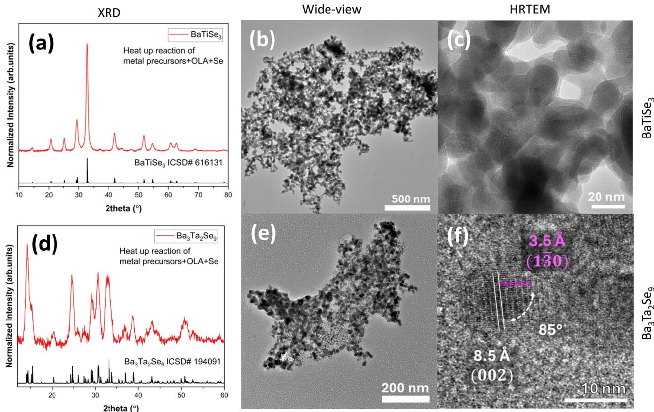
Fig. 6 Ba–M–Se nanocrystals synthesized via the methods discussed are shown here.  $\text{BaTiSe}_3$  is shown in (a–c),  $\text{Ba}_3\text{Ta}_2\text{Se}_9$  is shown in (d–f). The  $\text{BaTiSe}_3$  presented here was synthesized via the reaction method where elemental Se was heated up with metal precursors. Due to the significant aggregation and overlap of  $\text{BaTiSe}_3$  NCs in (c), we leave the visible lattice fringes unlabeled. An FFT analysis is provided in the SI for (c).
