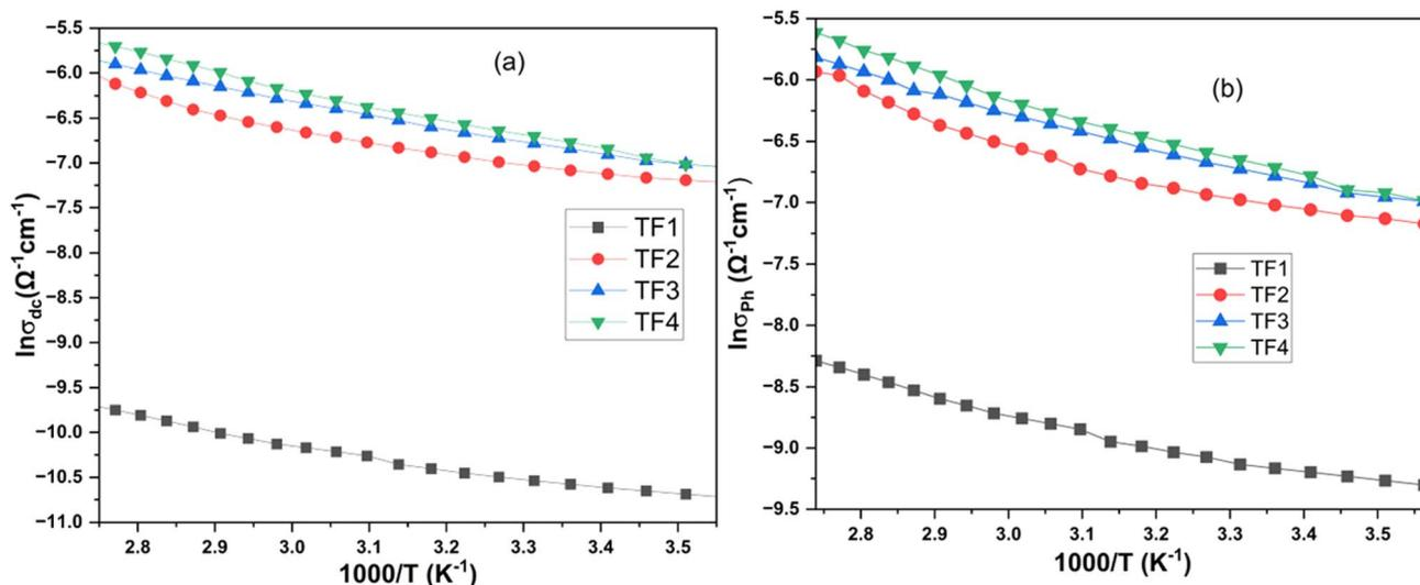
Fig. 4 DC conductivity and photoconductivity of the as-prepared (un-irradiated) and SHI-irradiated thin films of the  $(\text{Ga}_{10}\text{Se}_{90})$ -CNT composite. (a) DC conductivity: variation of  $\ln(\sigma_{\text{DC}})$  vs.  $1000/T$ . (b) Photoconductivity: variation of  $\ln(\sigma_{\text{Ph}})$  vs.  $1000/T$ .
