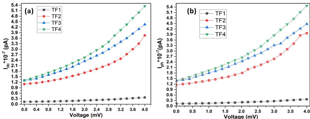
Fig. 3 Variations of the dark DC current and photocurrent with the applied voltage. (a) Dark DC current *versus* voltage, and (b) photocurrent *versus* voltage of the as-prepared and SHI-irradiated thin films of  $(\text{Ga}_{10}\text{Se}_{90})\text{-CNT}$ .
