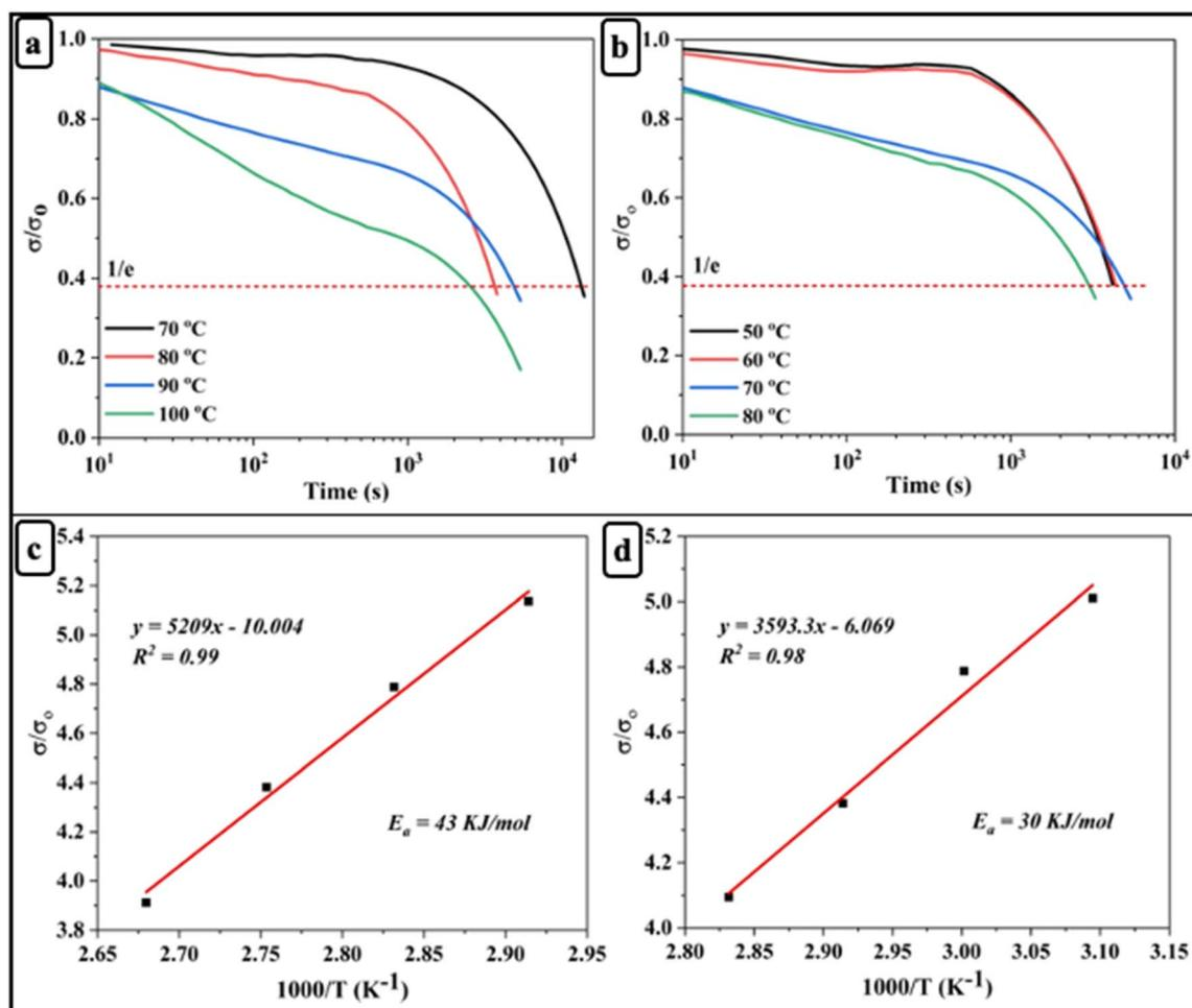
Fig. 3 (a) Stress-relaxation for D70B30; (b) stress-relaxation for D50B50 at different temperatures; (c)  $\ln(\tau)$  versus  $1000/T$  plot for D70B30; (d)  $\ln(\tau)$  versus  $1000/T$  plot for D50B50 bio-based epoxy vitrimers.
