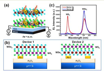
Fig. 1 (a) Schematic illustration of the dual-color electroluminescent device utilizing stacked monolayers of WS<sub>2</sub> and WSe<sub>2</sub> with independent AC-driven electrodes. (b) Cross-sectional schematics of Device 1 and Device 2. (c) EL spectra for both devices, showing emission from WS<sub>2</sub> and WSe<sub>2</sub>.
