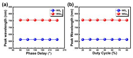
Fig. 4 Spectral stability for the dual-color EL device (a) phase delay dependent and (b) duty cycle dependent.
