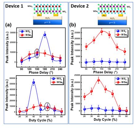
Fig. 3 EL peak intensity of WS2 and WSe2 as a function of phase delay (top) and duty cycle (bottom) for Device 1 (a) and Device 2 (b), highlighting tunable and balanced emission in Device 1 and persistent imbalance in Device 2. Error bars represent the standard deviation.
