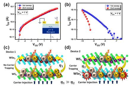
Fig. 2 Transfer characteristics for (a) WS<sub>2</sub> FET; inset: FET device structure. (b) WSe<sub>2</sub> FET. (c and d) Schematic representations of carrier injection and recombination processes in Device 1 and Device 2.
