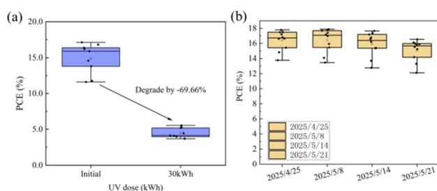
Fig. 9 (A) PCE degradation of MAPbI<sub>3</sub> perovskite sub-modules under UV accelerated ageing with a total dose of 30 kWh m<sup>-2</sup>. (B) PCE change of the same modules after 25 days of outdoor exposure.
