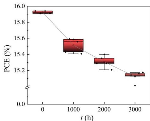
Fig. 8 Damp-heat accelerated ageing data for perovskite modules.
