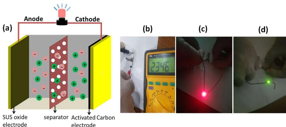
**Fig. 8** (a) The inner-side charge-storage mechanism of the fabricated device. (b) The recorded voltage of the device. (c and d) The different colors (red and green) of LEDs turned ON when connected to the device.
