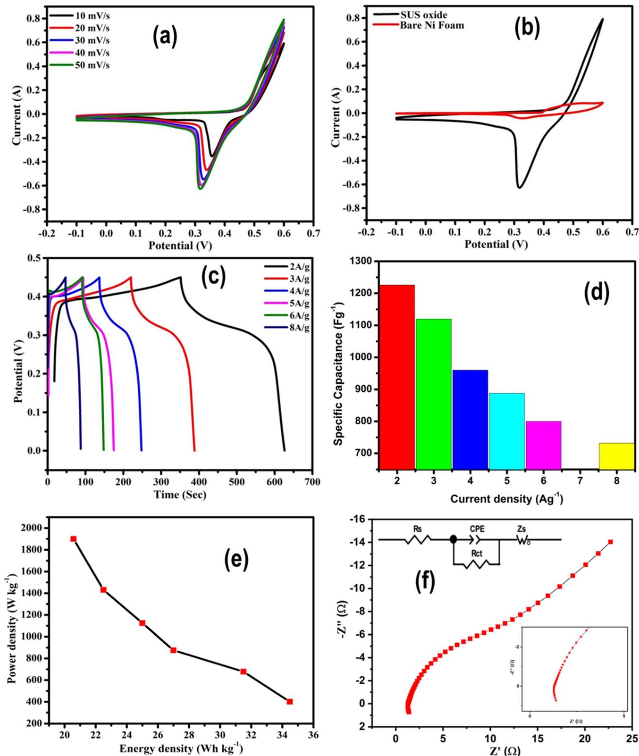
Fig. 6 (a) CV curves of the SUS-304L oxide at different scan rates (10–50 mV s<sup>-1</sup>) in a potential window of –0.1 to 0.6 V. (b) CV curves of the bare Ni-foam and SUS-304L oxide electrode at 50 mV s<sup>-1</sup>. (c) GCD curves at various current densities in the potential window of 1 to 0.5 V. (d) A graph of the capacitance vs. current density. (e) The cyclic stability graph. (f) The Nyquist plot at low and high magnifications.
