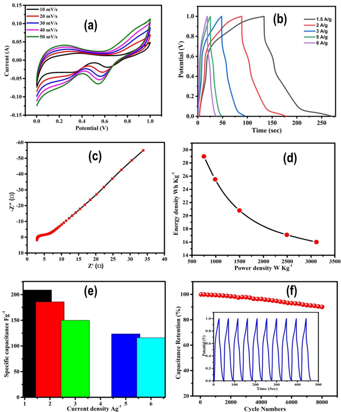
Fig. 7 (a) CV of SUS-304L oxide//AC at different scan rates ranging from 10–50 mV s<sup>-1</sup> in a potential window of 1 V. (b) GCD curves at various current densities in a potential window of 1 V. (c) Nyquist plot. (d) Ragone plot between energy density and power density. (e) Graph of capacitance vs. current density. (f) Cyclic stability of the fabricated device.
