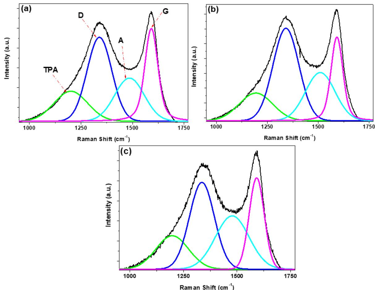
Fig. 4 Peak fitted Raman spectra of (a) SCS-B<sup>+</sup>, (b) SCS-N<sup>+</sup> and (c) SCS-Ne<sup>+</sup> samples after 7 h implantation times.
