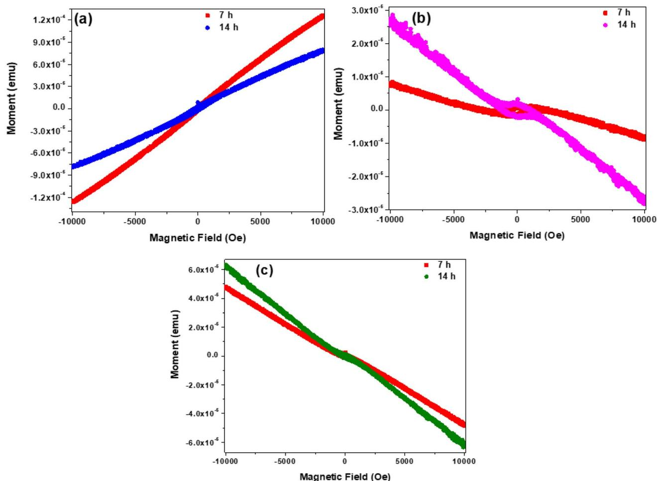
Fig. 8 Isotherm curves of the SCS-Ne<sup>+</sup> samples after different irradiation times at (a) 2 K, (b) 10 K and (c) 40 K.
