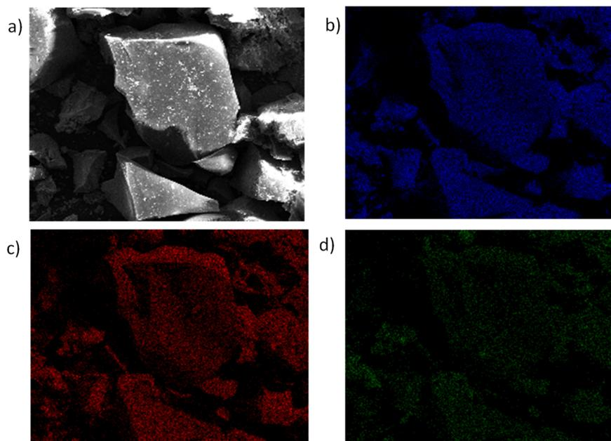
Fig. 9 Elemental mapping for  $\text{SiO}_2$ -ZnO composite annealed at 900 °C (a) the sample itself (b) Si (c) O (d) Zn.
