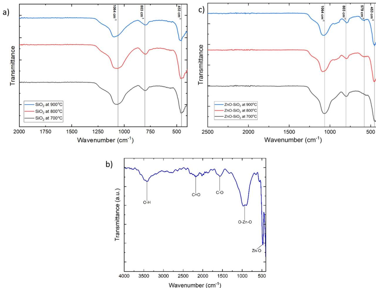
Fig. 4 FTIR spectra for (a) SiO<sub>2</sub> at 700 °C, 800 °C and 900 °C (b) ZnO at 450 °C (c) ZnO–SiO<sub>2</sub> composite at 700 °C, 800 °C and 900 °C.
