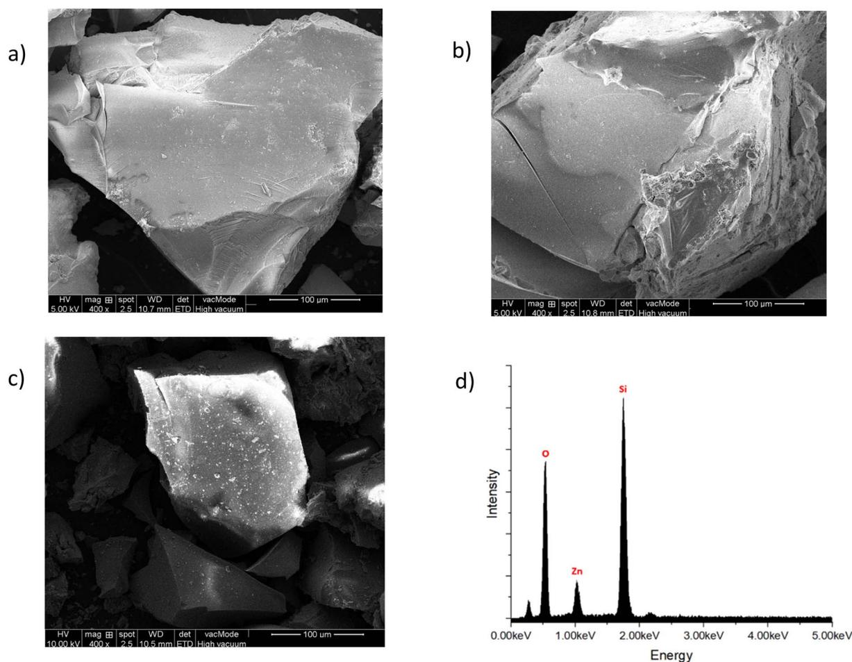
Fig. 8 SEM images of ZnO-SiO<sub>2</sub> composite at annealing temperatures (a) 700 °C, (b) 800 °C and (c) 900 °C (d) EDS spectrum of composite annealed at 900 °C. (d) EDS mapping of ZnO-SiO<sub>2</sub> nanocomposite 900 °C.
