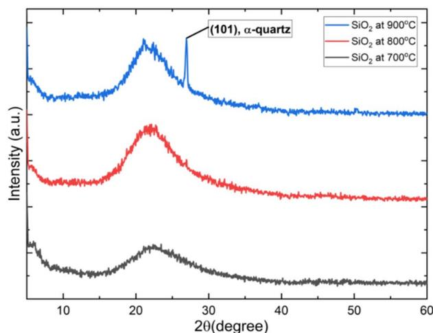
Fig. 1 XRD pattern for SiO<sub>2</sub> at different annealing temperatures.
