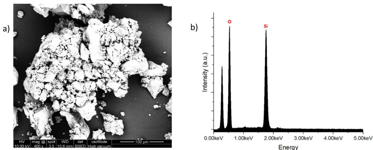
Fig. 6 (a) SEM image of SiO<sub>2</sub> annealed 900 °C (b) EDS mapping of SiO<sub>2</sub> annealed at 900 °C.
