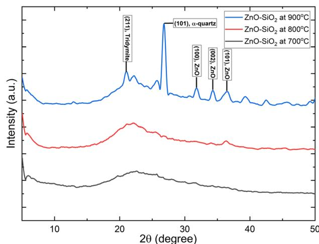
Fig. 3 XRD pattern for ZnO-SiO<sub>2</sub> composite at different annealing temperatures.
