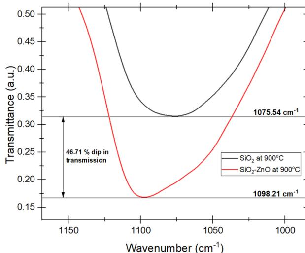
Fig. 5 Increase in absorption intensity on incorporation of Zn into the SiO<sub>2</sub> matrix.
