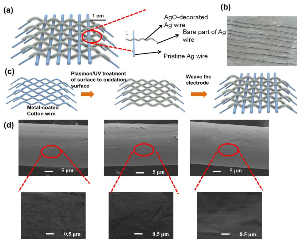
**Fig. 1** (a) Schematic illustration of an integrated all-silver memristor array. (b) Photo image of a all-silver memristor array. (c) Fabrication process of the memristor array. (d) SEM images of pristine Ag electrode (left panel) and Ag electrode after plasmon treatment (middle panel) and Ag electrode decorated with AgO by ALD (right panel).
